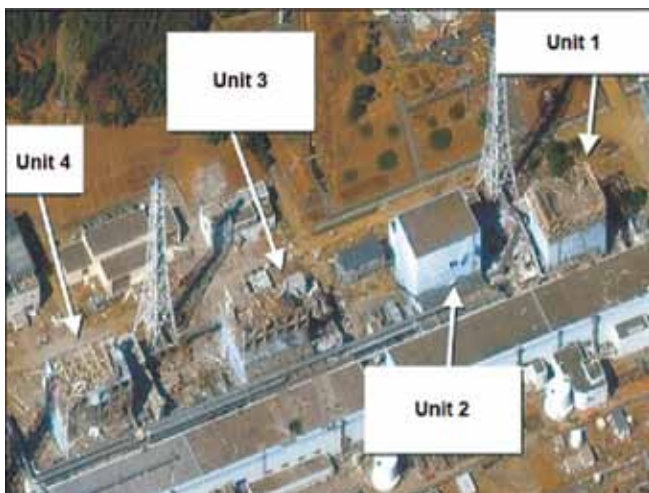
The emergency cooling generators were flooded leading to hydrogen explosions in the plant.
