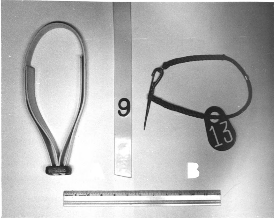
Figure 7. Plastic collars used for marking deer. A. Numbered plastic collar and buckle. B. Self-attaching poly-vinyl rope collar.
