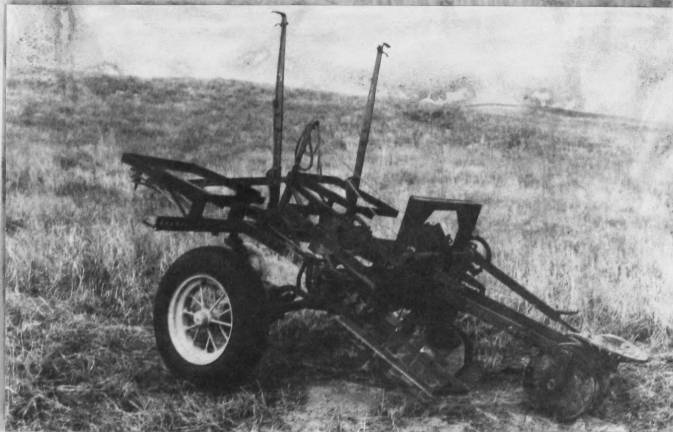
Fig. 8 Front and Rear Views of Nebraska Planter (Courtesy of U. S. Forest Service)
