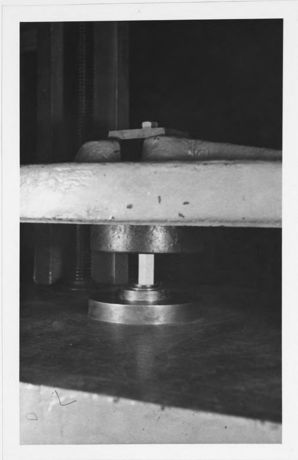
Figure 13.—Method of performing compression parallel to grain test.
