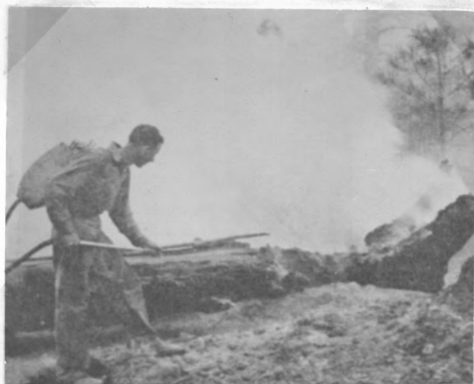
Fig. 4. Fire fighting with a back-pack bag and a trombone-type hand pump. (After a photo by the U. S. Forest Service).
