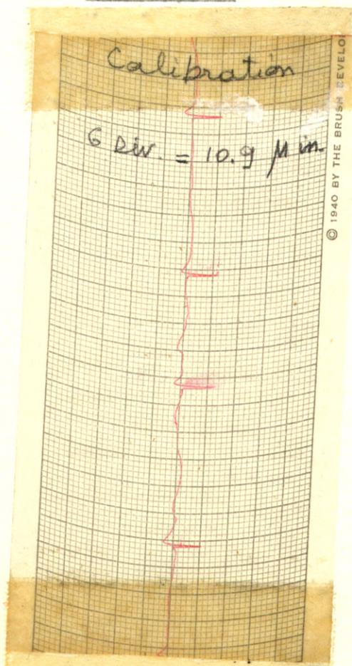
The analyser was calibrated by having the stylus ride on a perfectly smooth glass surface, containing however a small groove of known depth (10.9 micro in.); we can see on the chart at left that it corresponds to about 6 divisions on the graph paper used.
