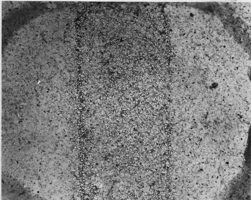
Figure 3. Band of hematite in Nugget sandstone from ridge south of Burbank Creek. (9.5 diam)
