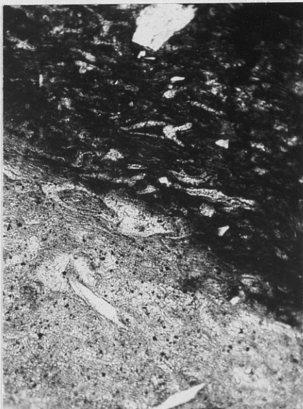
Figure 25. Boundary between pellet and groundmass. The lower, lighter portion of the photograph is the material of the pellet. (45 diam.)
