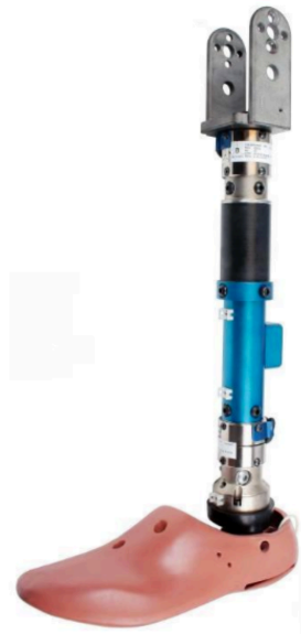
Figure 1. MIL-LX, which uses the midsize-male Hybrid-III foot (Humanetics Innovative Solutions).
