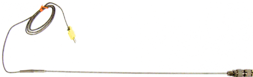
Figure 2.2: Proxy reactor with K-type 18 in. thermocouple
