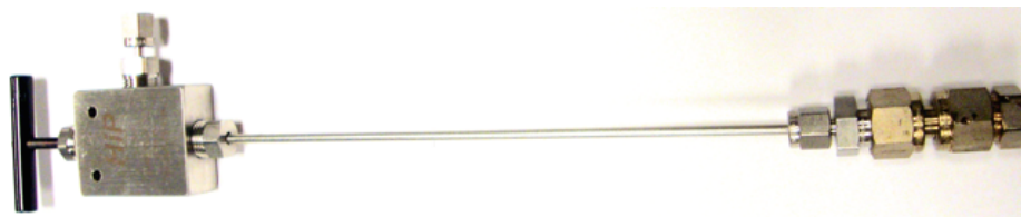
Figure 3.1: Reactor with gas valve assembly
