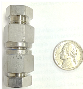
Figure 2.1: 1.67 mL mini batch reactor with U.S. nickel for scale
