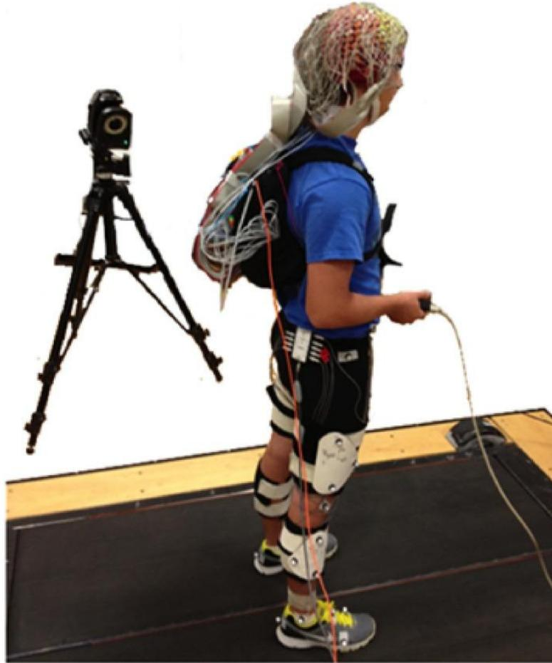
**Figure 2-1. Experimental Setup.** 20 subjects stood (0.0 m/s) and walked (0.4, 0.8, 1.2, and 1.6 m/s) on a treadmill while continuously performing the Brooks spatial working memory task. We recorded EEG, kinematics, ground reaction forces, and response data from the Brooks task.
