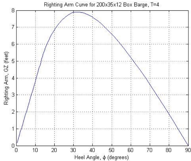
Figure 5-9 - Typical GZ Curve
