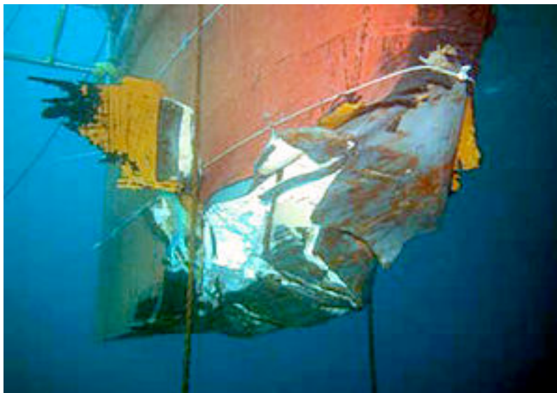
Figure 6.1. The damage to the USS Hartford after the accident 286
