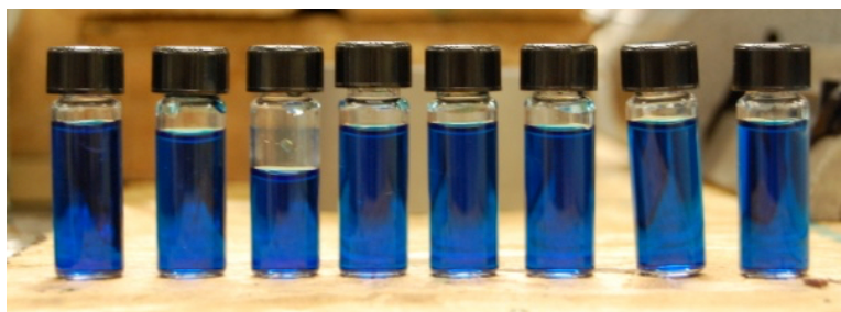
Figure 5.33: Samples of MB with PBS treated by plasma jet. Leftmost vial, t = 0 (before plasma treatment); rightmost vial, t = 5 minutes. Samples taken roughly every 45 seconds.
