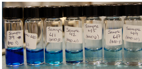
Figure 5.25: MB treated by microdischarge ( \sim 5 \text{ W} ). Samples range from t = 0 to t = 46 minutes of treatment time.
