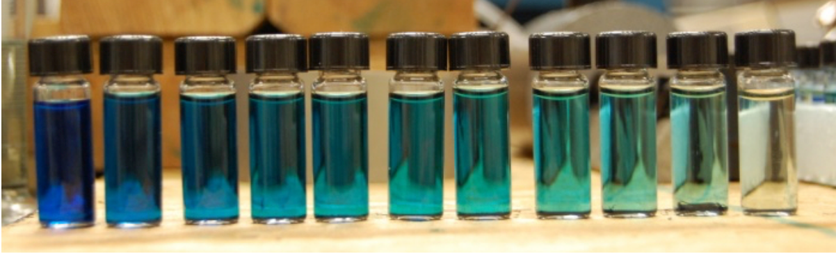
Figure 5.24: Samples of a methylene blue plasma jet decomposition trial, from t = 0 (leftmost) to t = 5.5 minutes (rightmost). Samples taken every 30 seconds, two rightmost samples taken 60 seconds apart [375]. \sim 4 \text{ kV}_{\text{pk-pk}} , 2 kHz, 1.65 SLPM flow rate of room air.
