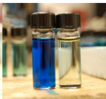
Figure 5.37: Comparison of MB solution with PBS (left vial, 5 min processing) and without (right vial, 5.5 min processing).
