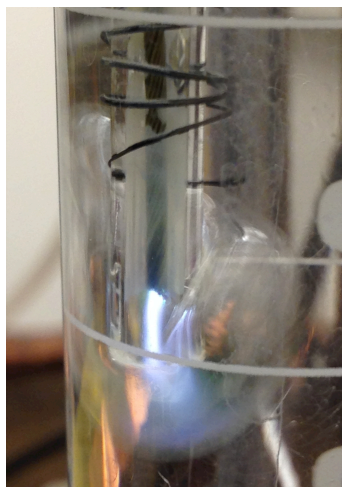
Figure 6.1: The steam discharge in operation.
