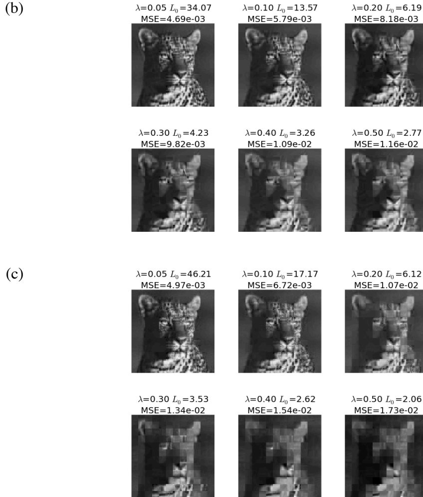
Figure 4.8: Image reconstructions using coefficients obtained from the LCA algorithm after different training implementations: (a) gradient descent, (b) WTA software implementation, (c) WTA using the device model.
