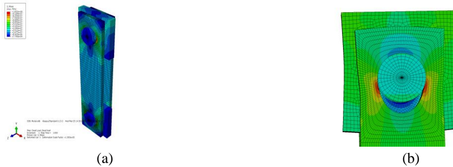
Figure 6-4. Link plate dead load validation testing showing (a) von Mises stress distribution and (b) pin hole deformation (largely exaggerated) with stress concentration
