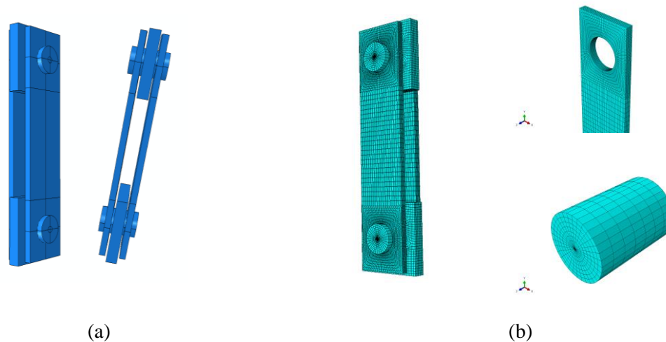
Figure 6-3. Link plate model (a) assembly and (b) meshing
