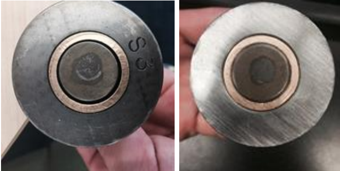
Figures 29 & 30: The fatigued bushing shown on the left shows significantly more wear than the new bushing on the right.
