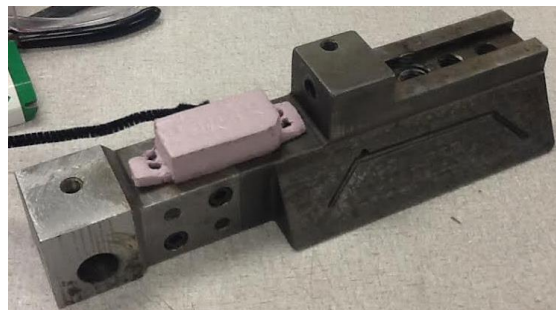
Figure 15: The foam mockup of the Wintriss strain link, to accurate dimensions, on top of a S3F slide.
