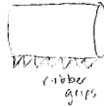
Figure A7: Foot pad with many small contact points for added friction
