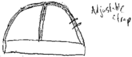
Figure A17: Flat pedal with adjustable strap
