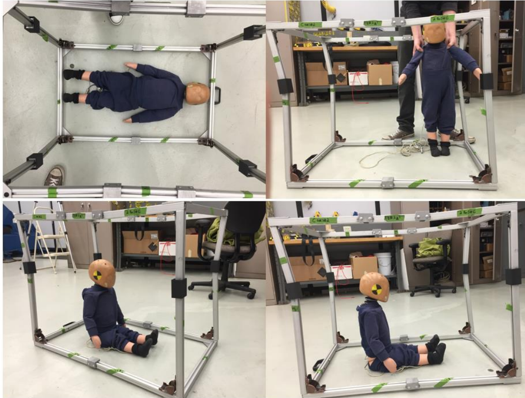
Figure 22: 95th percentile 18 month old anthropomorphic test dummy inside of our prototype
