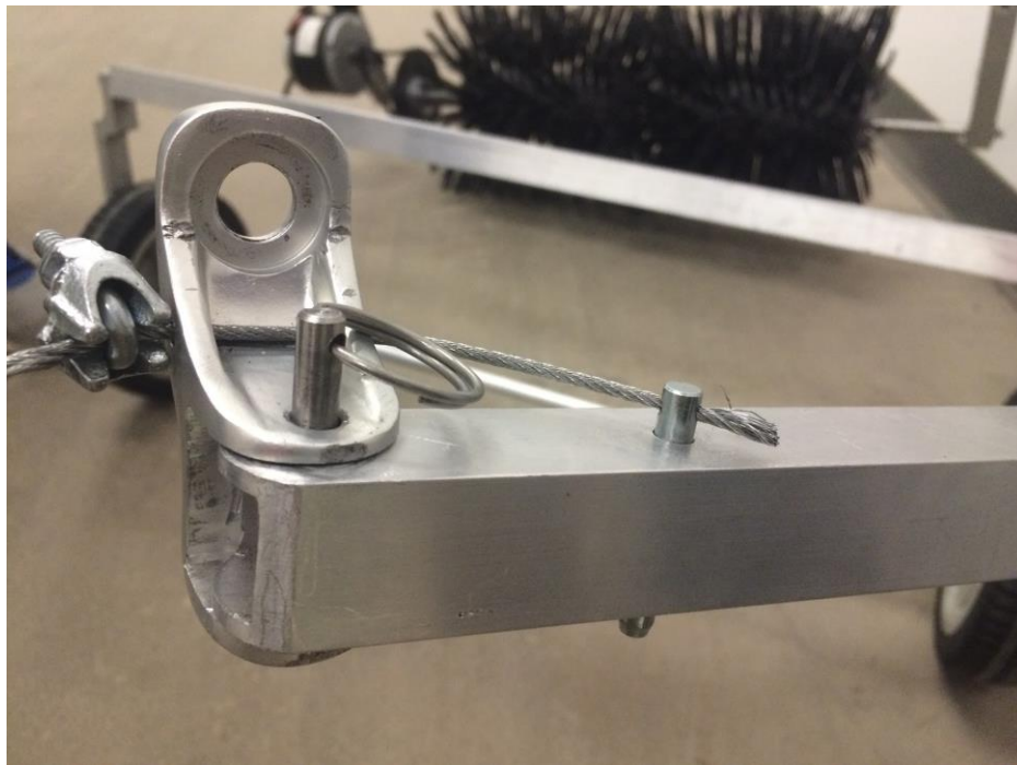
Figure 22: Steel Cable to Eliminate Excessive Device Rotation
