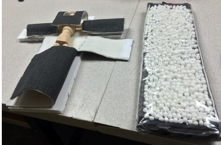
Figure 17: Mockups of both resistive (left) and conductive-bead (right) heating methods. [Personal photograph by Ben Lewis. 1 Oct 2015.]
