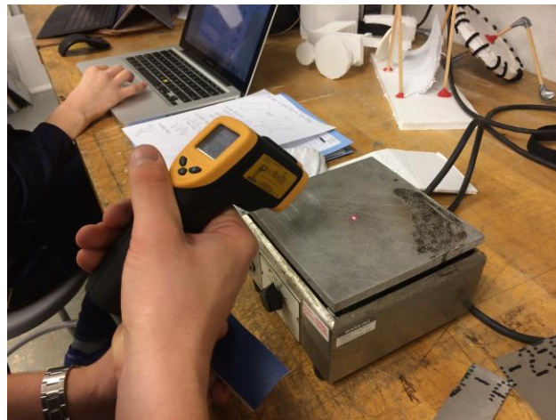
Figure 23: Experimental test using hot plate, Al sheet and polyurethane coated nylon fabric. [ Personal photograph by Ben Lewis. 20 Oct 2015. ]
