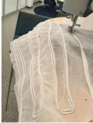
Figure 40: Stitching the wires into the cotton/porous-fabric.
