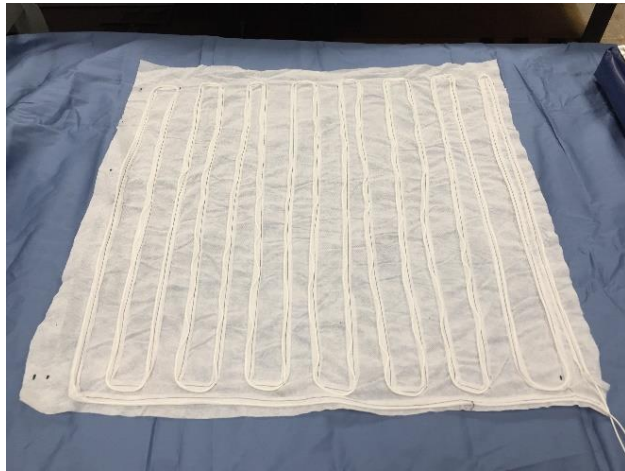
Figure 41: Completion of the evenly sewn heat source (snake-like pattern).
