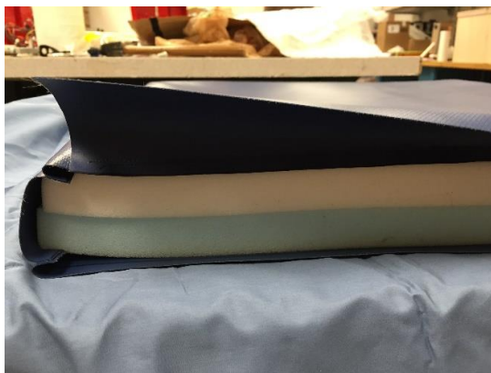
Figure 47: Cross section of device before completely sealing.
