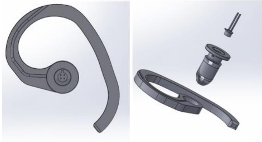
Figure 39: Exploded view of the ear clip, ear bud, and infrared thermometer used to measure core body temperature at the tympanic membrane [74].
