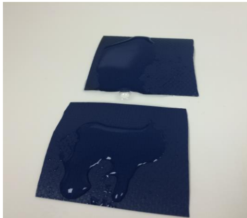
Figure 21: Polyurethane coated nylon fabric samples with 1:10 bleach solution pooled on surface. [ Personal photograph by Ben Lewis. 20 Oct 2015. ]
