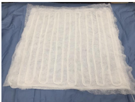
Figure 46: From bottom to this top view: two foams, deflector, embedded wires, and thin cotton overlay.
