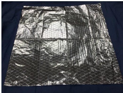
Figure 42: The deflector, used to prevent heat loss the bottom of the OR bed.
