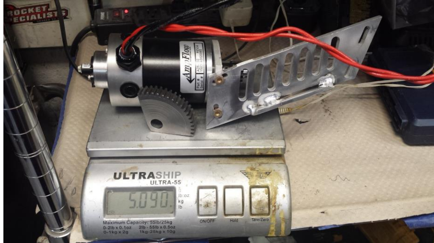
Figure 35: The weight of the system is below 6 lb, meeting the user requirement.
