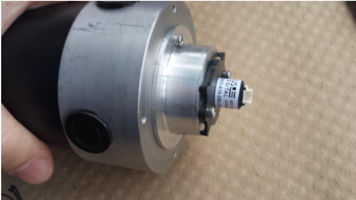
Figure 40: New encoder mount is installed properly onto the motor.
