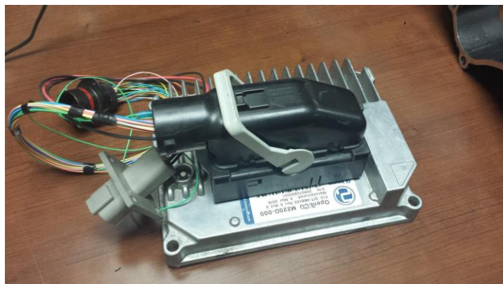
Figure 8: A mock-up of a Pi Innova M220 controller was not produced because the sponsor was able to lend a spare model that they had on hand. Below is a picture of the controller that will be used.
