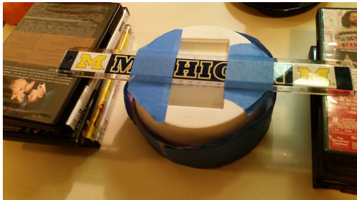
Figure 25: Two-piece mold fully assembled
