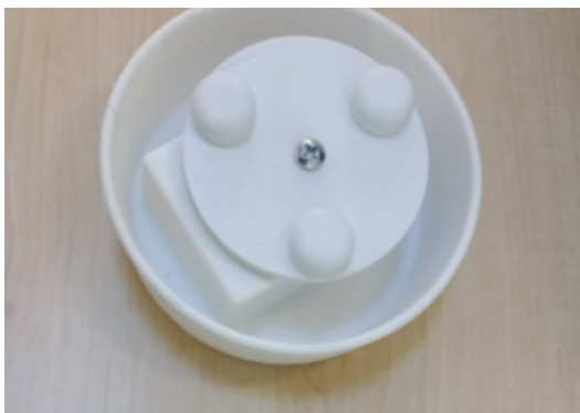
Figure 22: 3D printed turning plate and housing, viewed from the bottom.
