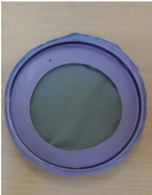
Figure 26: Silicone covering (purple) with nylon insert (green)
