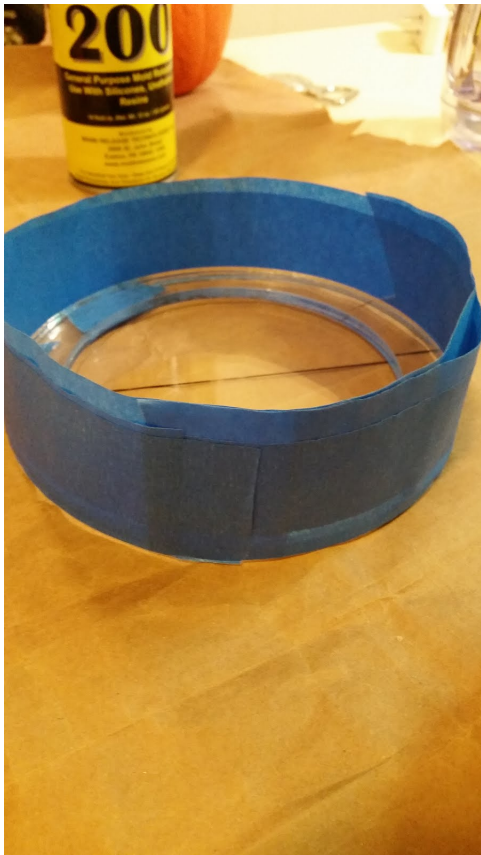
Figure 23: Part one of the two-piece mold
