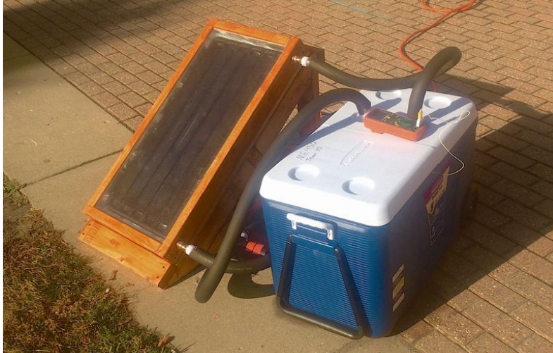
Figure 18: This is the testing set-up including the thermocouple used to determine the reserve tank temperature.
