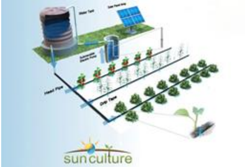
Figure 1.2: SunCulture solar-powered irrigation system [4].
