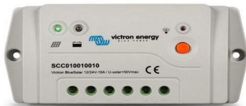
Fig. 5.3: Example of solar charge controller [28]
