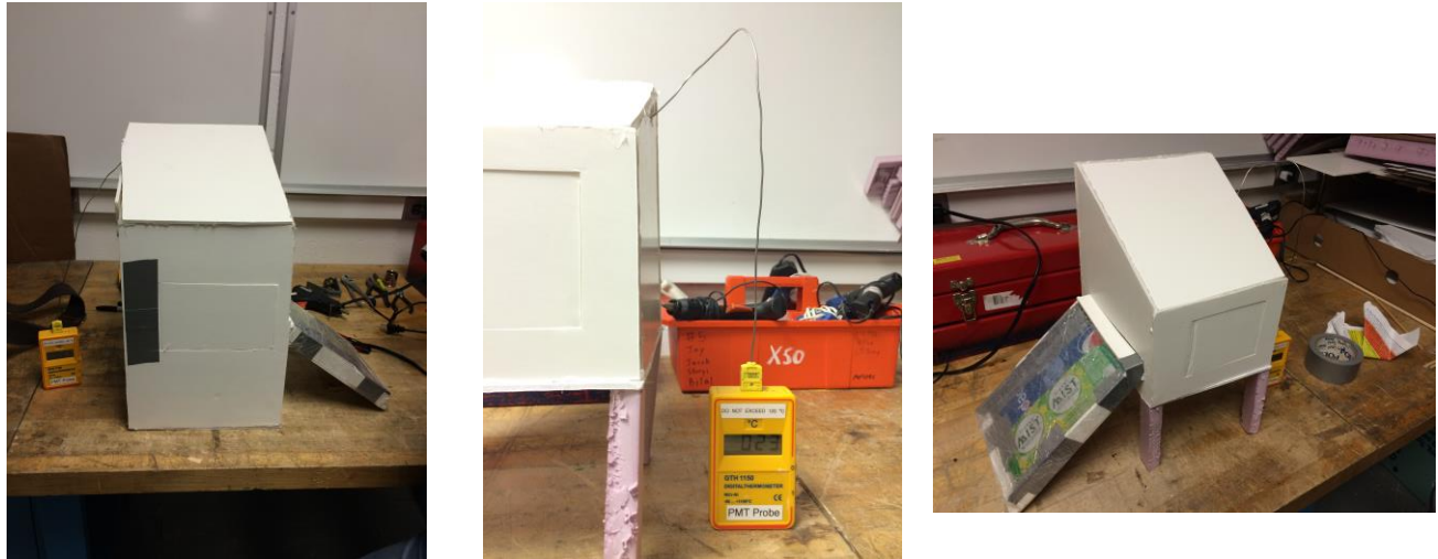
Figure 20: Testing of sand as additional heat mass for drying chamber. Results showed slower heat-up time with addition of sand.
