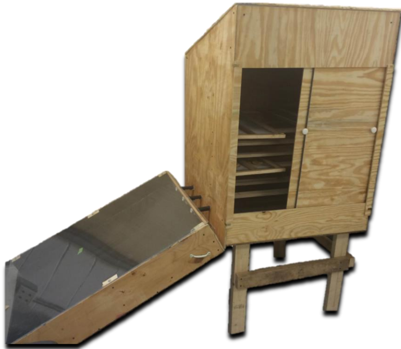
Figure 16: Manufactured first prototype of fruit dryer. Support cross-bars were included to the legs for additional stability.
