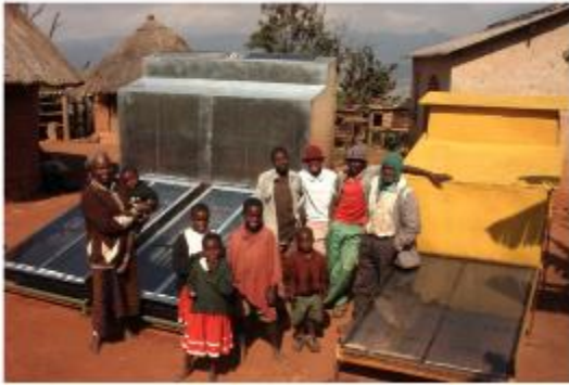
Figure 4 shows the indirect solar dryer to help dry fruit and coffee in Zimbabwe [8]. This dryer uses custom metal framework and solar panels which is too expensive for our desired design.
