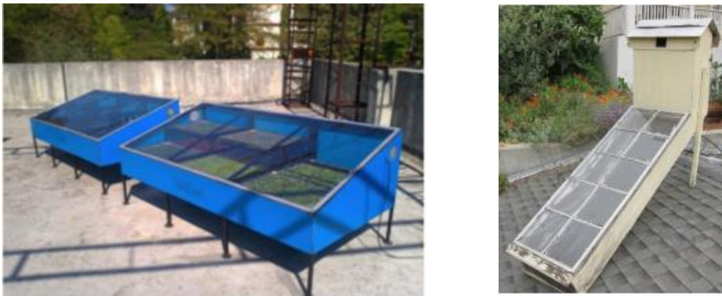
Figure 3: direct (left) and indirect (right) solar dryers. Direct utilize an open surface for the sun to directly shine on the fruit, while indirect relies on heated, dry air to dry the fruit instead of sunlight. [7]
