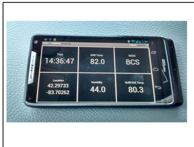
Figure 4 – DataProbe Screen Example in Phone, Surface Patrol, and CAN Mode
