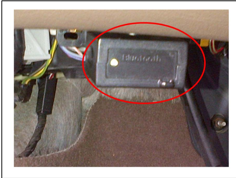
Figure 6 – Bluetooth enabled OBD Key for CAN data
