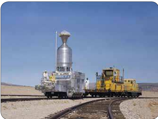
The Phobos 2A Nuclear Rocket
