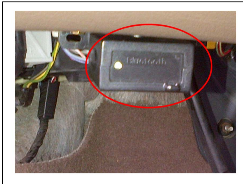
Figure 14 – Bluetooth enabled OBD Key for CAN data
