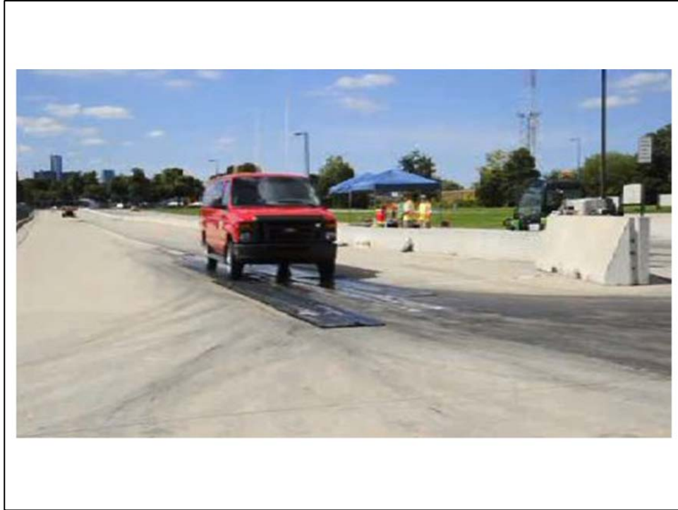
Figure 10 – Slippery Road Simulation on IMO Test Loop
