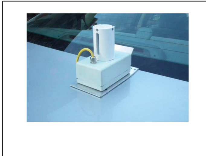
Figure 16 – Surface Patrol Humidity Sensor Mounted on a Car Trunk
