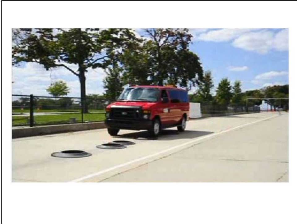
Figure 9 – Rough Road Simulation on IMO Test Loop
