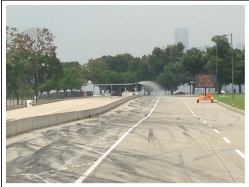
Figure 7 – Rain Simulation on IMO Test Loop
