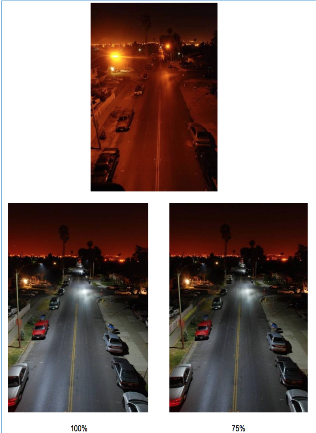
Figure: San Jose comparison of LPS and dimmable LED streetlights at 100% and 75% power. 163
