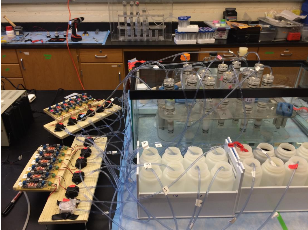
Image 2: iTIE laboratory system set up, with view of the iTIEs in the aquarium with test water, the peristaltic pump system, and the collection bottles, all connected via tubing (Kathryn Meyer, 2016)
