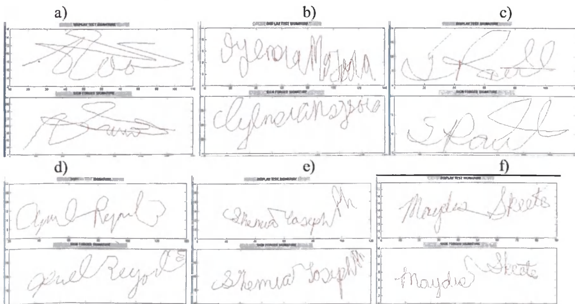
Figure 4.4.5 Single signature analysis for I-Pen input device a,b,c) Examples of rejected signatures d,e,f) Examples of accepted signatures
