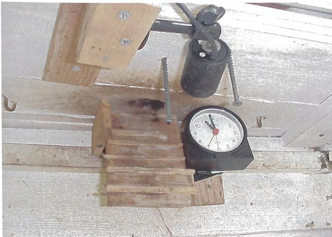
Figure 1- Single exit/entry portal located on the underside of a 30 cm false eave, 5 m above ground level. A standard infrared LED camera was mounted 15 cm forward of the entrance ramp, focused on the portal and an analog clock, 7 cm in diameter. See additional details in text.
