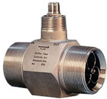
Figure 16. Inline turbine flow meter (Hoffer flow controls, Inc., Model HO 1/2X1/4A) and flow rate indicator
