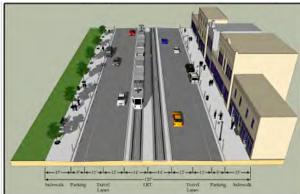
Figure 1: Cross-Section of Operating Option A: Median-Running/Traffic Separated Source: Woodward Light Rail Project and Parsons Brinkerhoff 2010 (Woodward Light Rail Project 2011)
