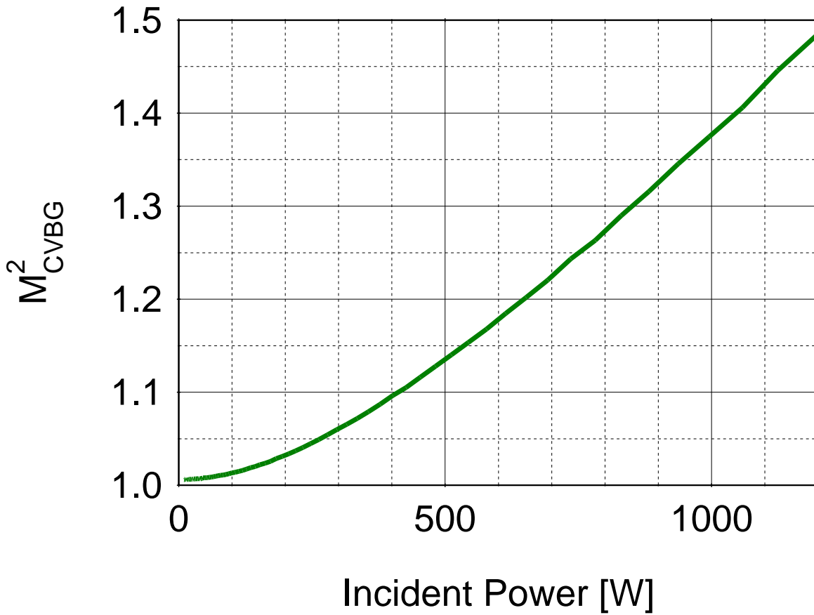
Figure 3.11 Calculated M^2 vs. input power for 2.7 cm long and 10 nm bandwidth CVBG.
