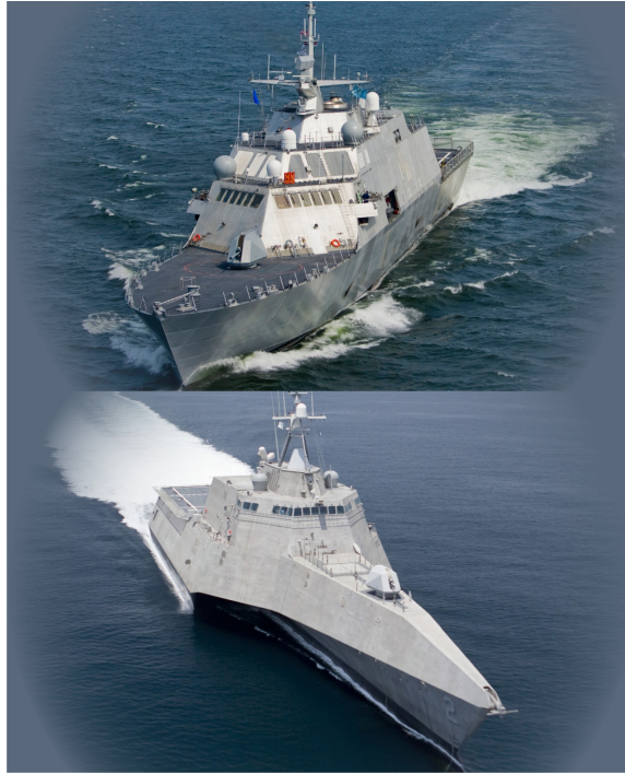
Figure 2.1: The two LCS variants. The top is the Freedom class steel-hulled monohull LCS built by Marinette Marine in Wisconsin, while the bottom is the Independence class aluminum hulled trimaran LCS built by Austal USA in Alabama. (US Navy, 2010)
