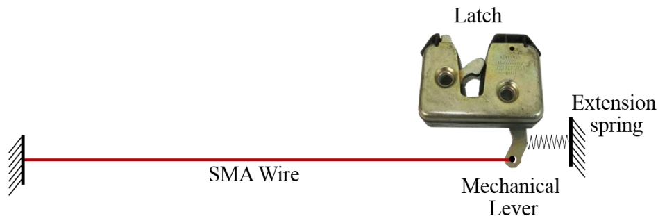
Figure 1.7. Latch release device.
