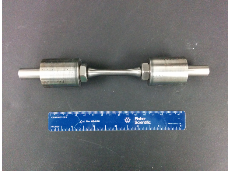
Figure 2.3: Assembled tensile and TMF specimen and superalloy extensions.
