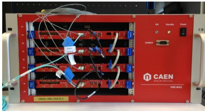
Fig. 4-8. CAEN VME crate containing 4 V1720 digitizers connected for time synchronization.
