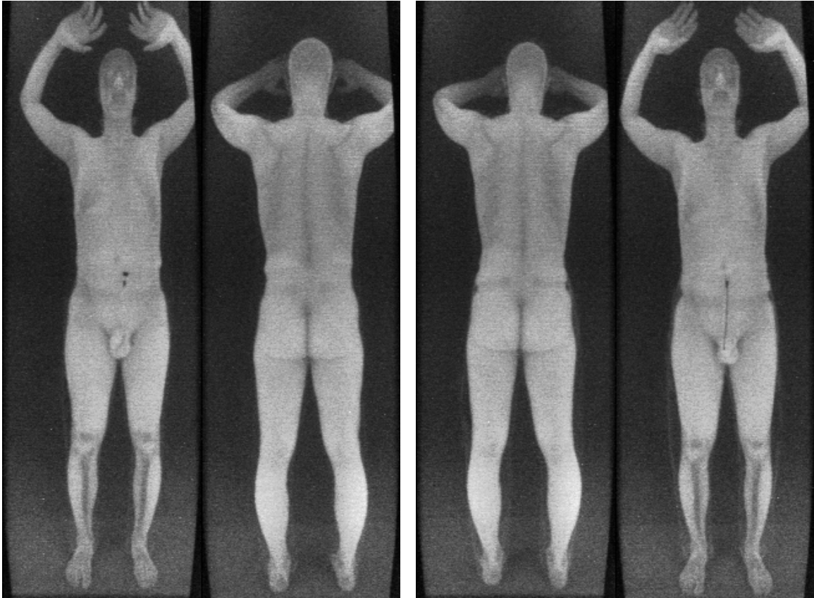
Figure 3.4: Concealing a Pistol by Positioning —The Secure 1000 cannot distinguish between high Z_{eff} materials, such as a metal handgun, and the absence of a backscatter response. Carefully placed metallic objects can be invisible against the dark background.
