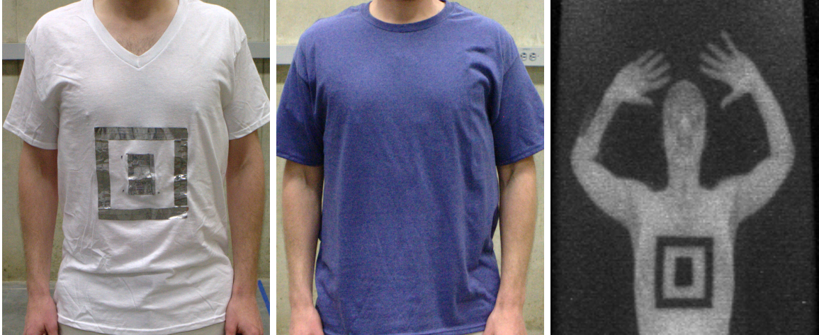
Figure 3.7: A Secret Knock —We demonstrate how malware infecting the Secure 1000 user console could be used to defeat the scanner. The malware is triggered when it detects a specific pattern in a scan, as shown here. It then replaces the real image (c) of the attacker, which might reveal hidden contraband, with an innocuous image stored on disk. Pattern recognition occurs in real time.
