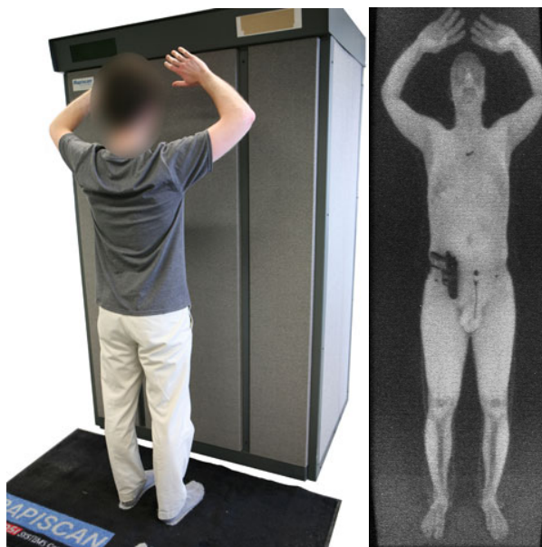
Figure 3.1: The Rapiscan Secure 1000 full-body scanner uses backscattered X-rays to construct an image through clothing. Naïvely hidden contraband, such as the handgun tucked into this subject’s waistband, is readily visible to the device operator.
