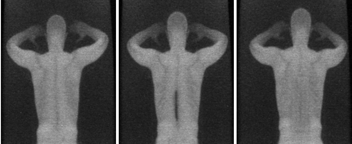
Figure 3.5: Concealing a Knife by Masking —We find that high- Z_{eff} materials can be hidden by covering them with lower Z_{eff} materials, such as the common plastic PTFE (Teflon). For example, a metal knife is clearly visible when naïvely concealed, but when covered with a thin plastic block it approximates the color of the spine. Tapering the block’s edges would reduce the visible outline.
