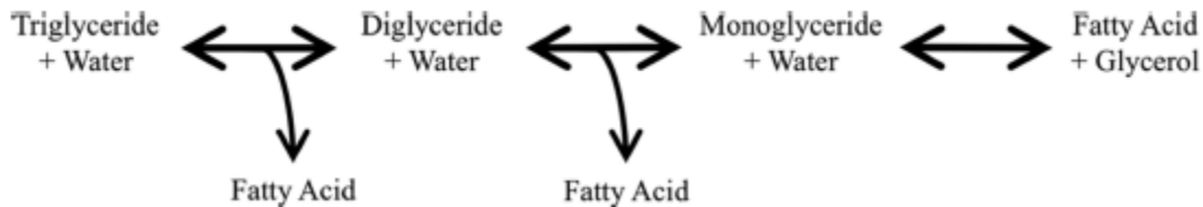
Figure 2.1: Reaction network for acylglyceride hydrolysis in hydrothermal condition [33]
