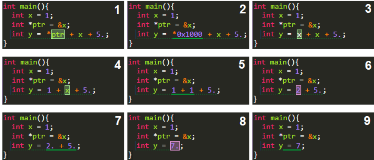
Figure 7.1: An example of expression evaluation visualized in Labster. Frames are shown top to bottom, left to right. The next operation to be performed is highlighted or underlined. Light green boxes indicate lvalue-to-rvalue conversions, whereas pink boxes indicate implicit arithmetic conversions.
