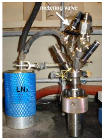
Figure 3.5 Reactor vessel and the Schlenk line setup to collect volatile products. Adapted from [4], supporting information.
