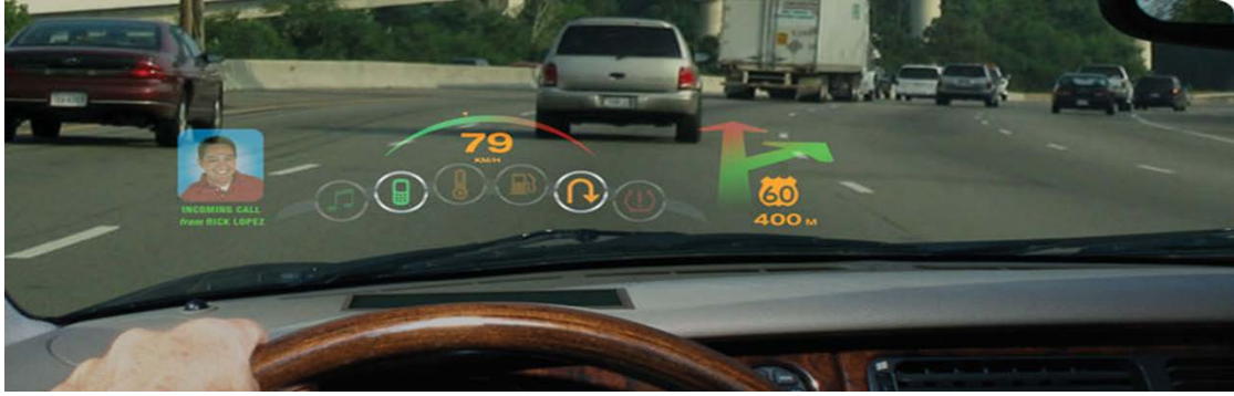
Fig. 7.1 Heads-up display where visible lasers are used to project the drivers speed and directions on the windshield [143].
