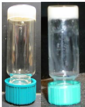
Figure S2.14 Gelators in a 4 mL vial (a) 3 in acetone/H 2 O (5:1) (b) 8 in MeOH/H 2 O (1:1).
