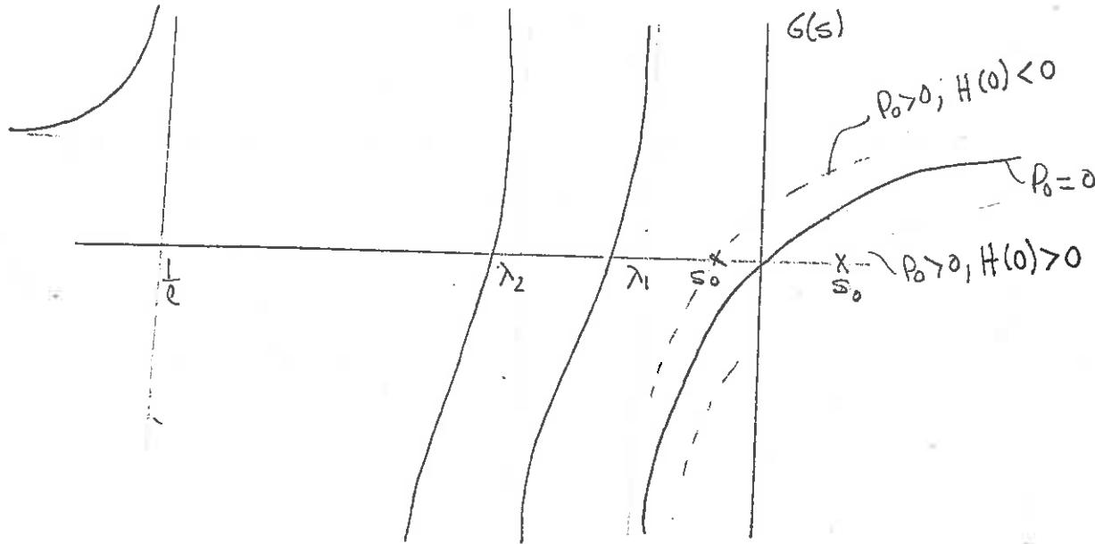
Note now that for a small, positive value of  $P_0$ , the curve shifts up or down depending upon the sign of the steady-state power coefficient
