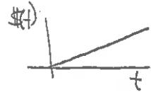
a.) Constant delayed neutron production rate approximation
