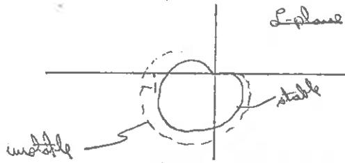
*Proof.* Consider the function  $\mathcal{L}(s) = 1 - P_0 H(s) Z(s)$ . It is a well-known theorem in complex variable theory that if  $\Gamma$  is a closed contour of  $\mathcal{L}(s)$  along a fixed direction  $\Gamma$  is  $2\pi$  times the number of zeros of  $\mathcal{L}(s)$  minus the number of poles of  $\mathcal{L}(s)$ .
