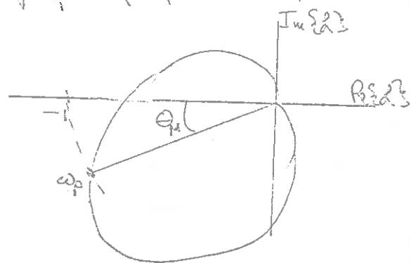
Frequently one must make do with a system having desired margins, and, if the system is stable with just desired margins, then the system is stable with them. But one must be careful since going over to non-minimum phase in which desired margins ordinary tends to decrease the stability of the system.
