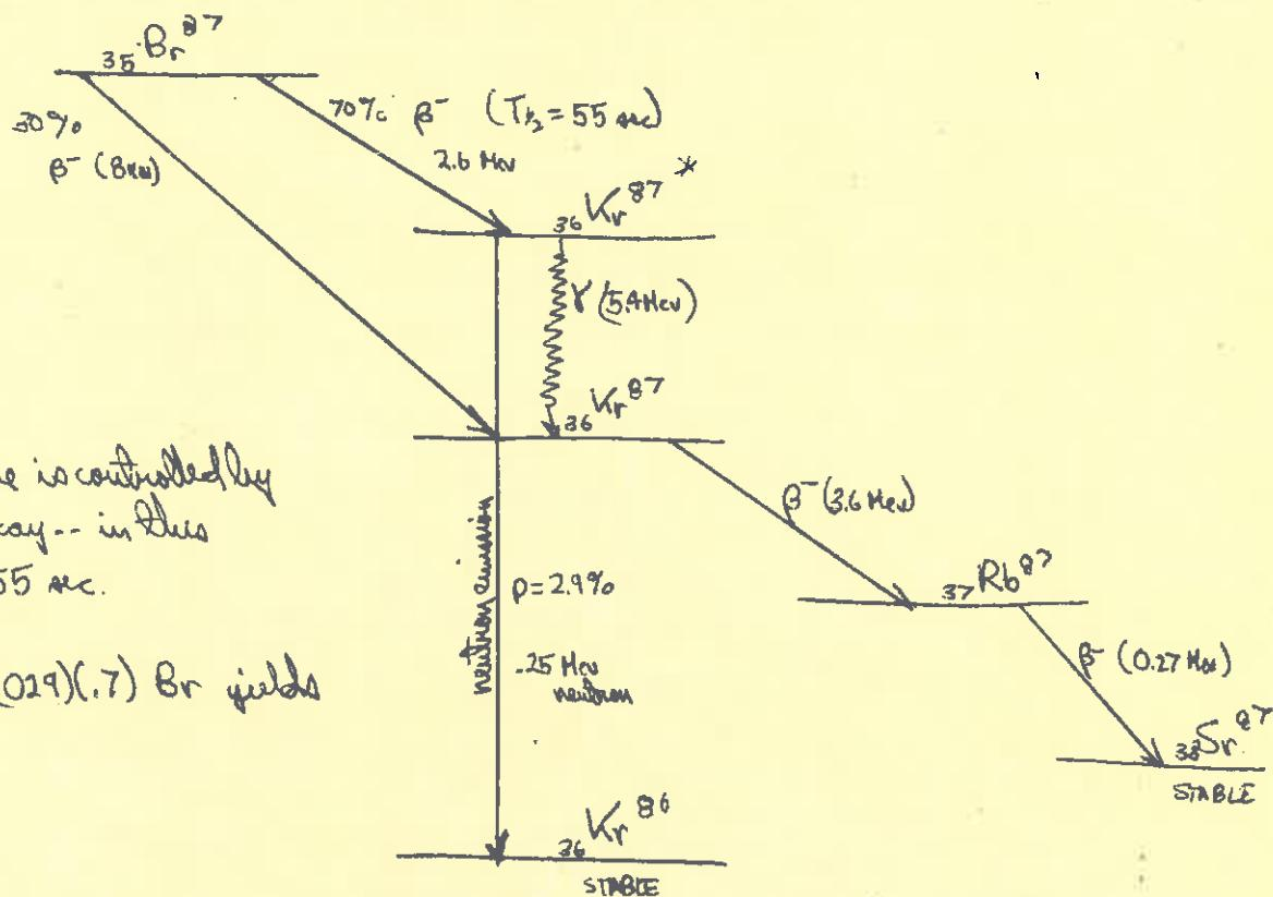
i.) Effective lifetime is controlled by preceding  $\beta$ -decay -- in this case,  $T_{1/2} = 55 \text{ sec}$ .
