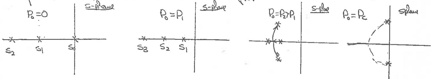
For some sufficiently large  $P_0$ ,  $s_0$  will encounter  $s$ , and form a complex conjugate pair. For still larger  $P_0$ , this pair moves back to the right, until for some critical power  $P_0 = P_c$ , the roots move into the RHP and the system becomes unstable. When the poles cross the imaginary axis, we perceive a "resonance" in the transfer function gain. (as we mentioned earlier).
