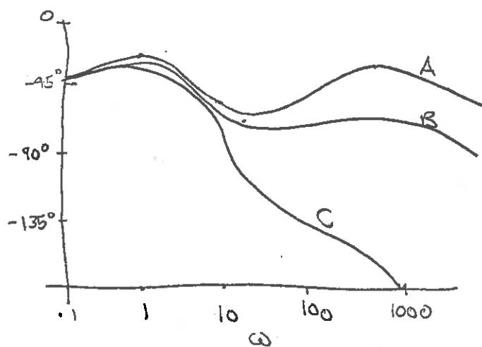
These measurements reveal the spatial dependence of the transfer function -- and, in fact, the breakdown of the P.R.K.E. Recall that in our consideration of these equations, we have been assuming that the shape function  $\Psi(r,v,t)$  in
