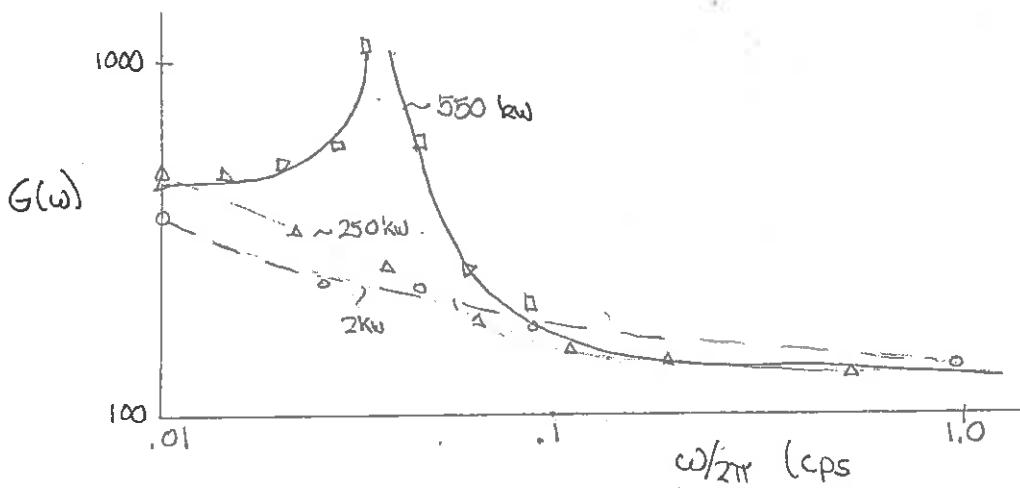
In particular, notice how different the transfer function of power is from the zero power transfer function. The mode resonance behavior in the vicinity of 0.03 cps at  $P_0 = 550$  kw is apparent. Such behavior
