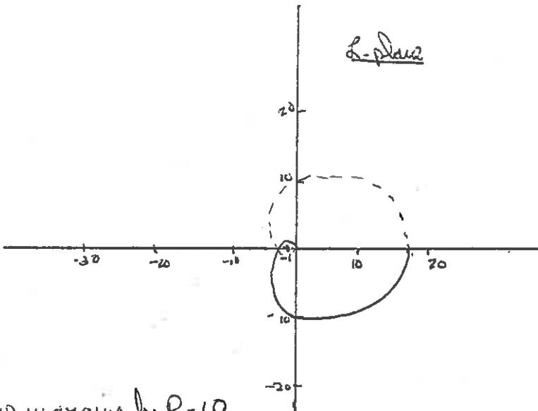
One can estimate the gain and phase margins for  $P_0 = 10$  either graphically or analytically.
