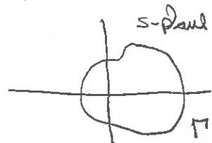
Since we wish to determine if  $\arg \mathcal{L}(s)$  has any zeros in the RHP, we need only apply this theorem along the indicated contour in the  $s$ -plane [ $s \rightarrow \infty$ ].
