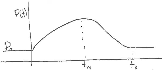
Then in fact we can demonstrate that the reactivity is negative at the time  $t_o$  when the power returns to its initial value  $P_0$ .
