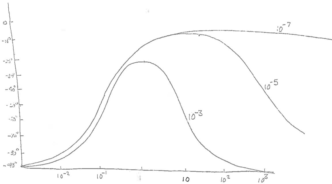
These figures are called "Bode diagrams". Note in particular that we have plotted the amplitude in  $\text{deg}$
