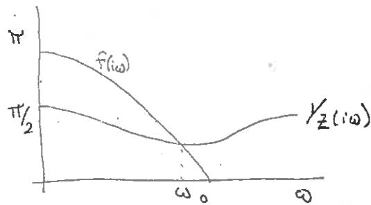
We can examine in more detail  $Y_Z(i\omega)$ . In fact one can show  $Y_Z(i\omega)$  has always in upper right quadrant of complex plane. Thus for instability to be possible, the feedback function  $H(i\omega)$  must lie in the same quadrant. Hence necessary conditions for stability are
