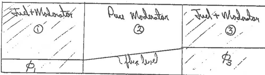
Suppose there is a control system keeping the total power of all three regions a constant (although the flux or power in an individual region is not constant).
