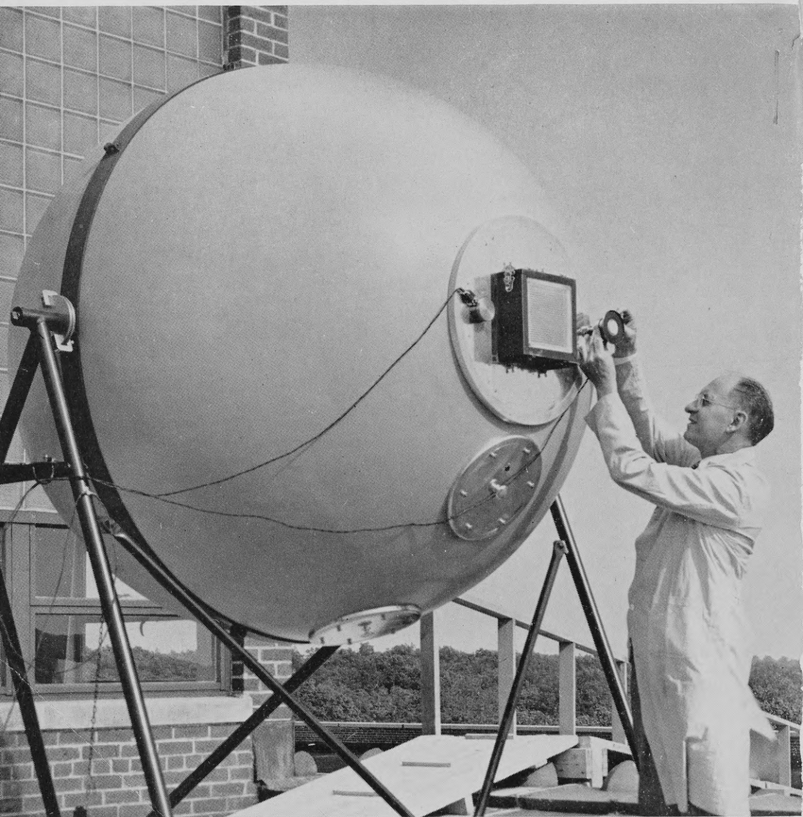
Integrating sphere, special engineering research
