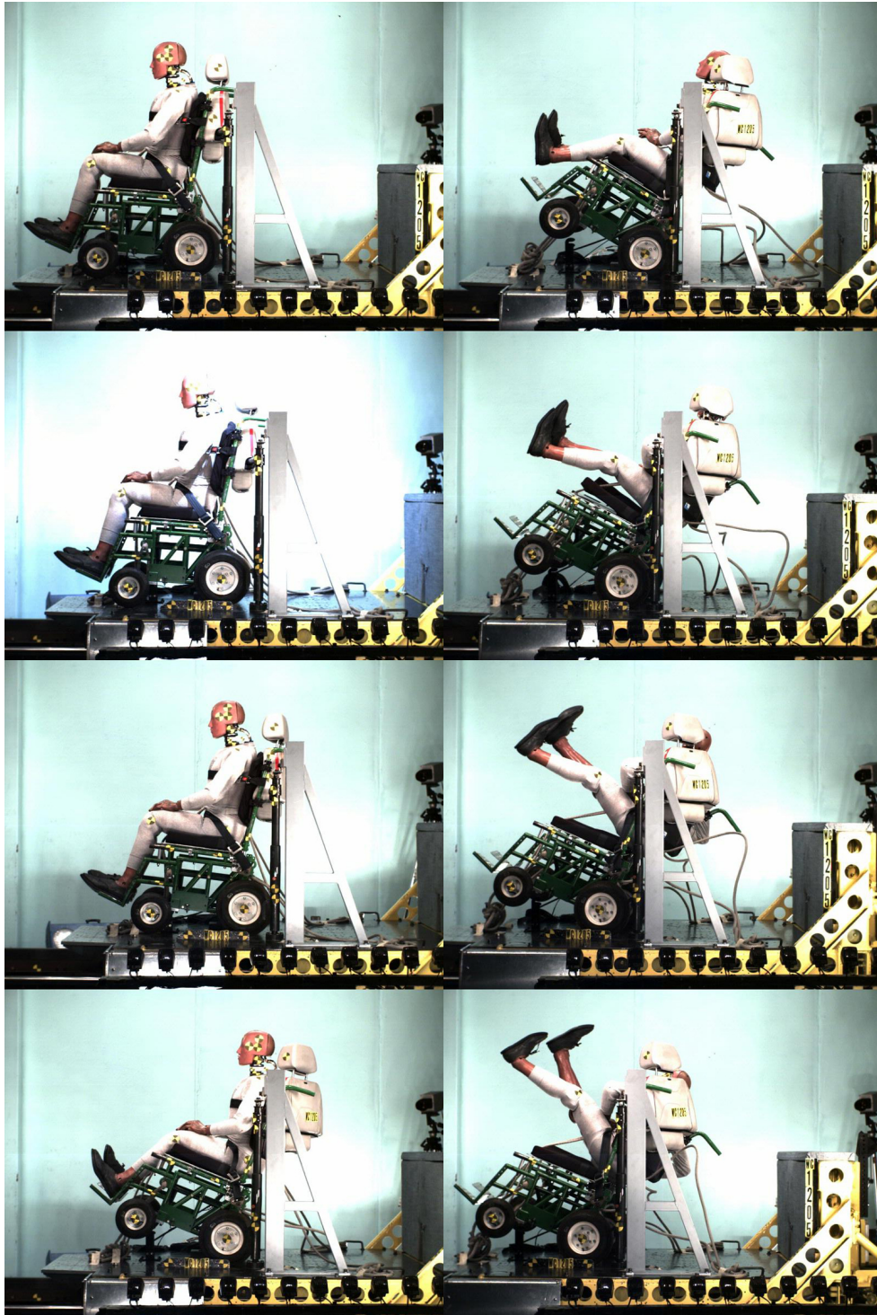
Figure 2.68 – Time-sequence frames from the side-view high-speed digital video of the second rear-impact sled test of the Swedish deployable vehicle-anchored head-and-back restraint system – note the rearward rotation of the SWCF
