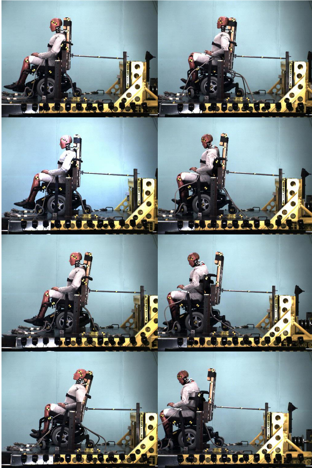
Figure 2.62 – Time-sequence frames from the side-view high-speed digital video of the second rear-impact sled test of the BME student-designed vehicle-mounted head-and-back restraint
