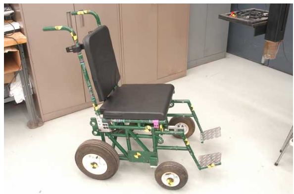
Figure 2.17 - Surrogate wheelchair frame (SWCF) used in tests to evaluate front- and rear-impact restraint systems to evaluate restraint systems in both front and rear impacts
