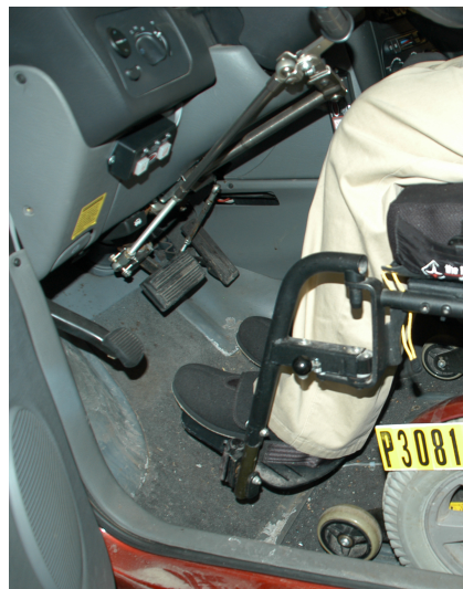
Figure 2.5 – Photo showing driver's knee position relative to the knee restraint and hand-control linkages
