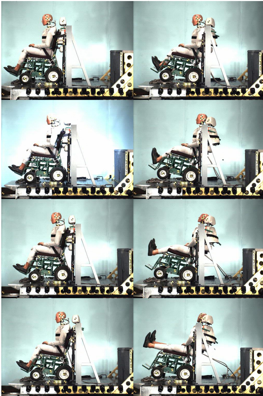
Figure 2.75 – Time-sequence frames from the side-view high-speed digital video of the fourth rear-impact sled test of the Swedish deployable vehicle-anchored head-and-back restraint system – note that there is no rearward rotation of the SWCF
