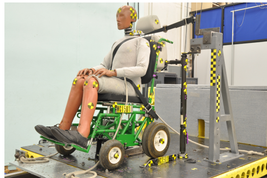
Figure 2.77 - Pre-test photos of the manufacturer’ revised design of the Swedish deployable vehicle-anchored head-and-back restraint system
