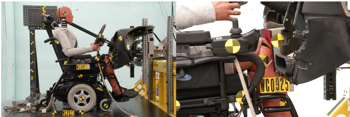
Figure 2.36 - Photos of the setup for frontal-impact sled test of the close-proximity knee restraint with no airbag and a two-point vehicle-anchored shoulder belt
