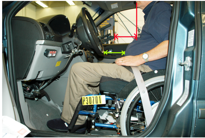
Figure 2.4 – Photo showing horizontal and vertical distances measured between the driver and the steering wheel and the steering assist device
