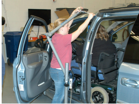
Figure 2.3 - UMTRI investigator taking measurements of a vehicle using the FARO Arm
