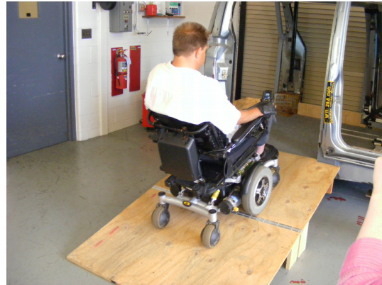
Figure 2.14 -Minivan buck in UMTRI high-bay laboratory with rear-entry and side-entry ramps used for wheelchair driver ingress and egress to evaluate prototype restraint-system designs
