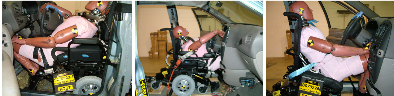
Figure 2.19 - Typical post-test positions of the ATD following TRC wheelchair-driver sled tests
