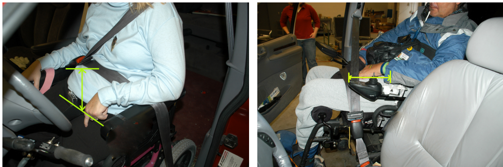
Figure 2.10 - Photos showing lap-belt locations over the arm supports and on the abdomen (left) and forward of the thigh-pelvis junctions (right)
