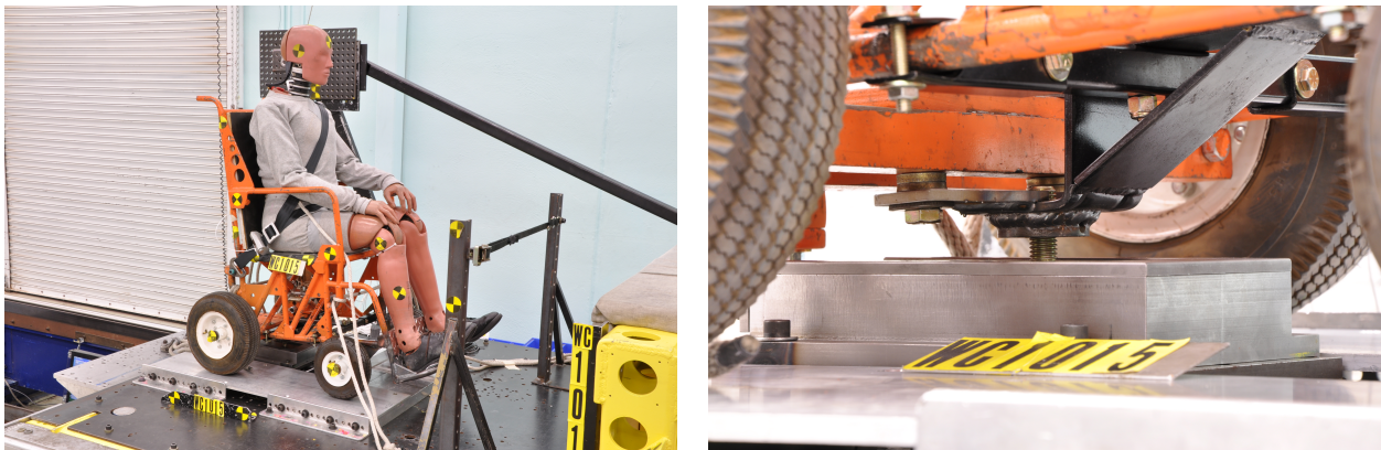
Figure 2.44 - Setup photos for a test of the surrogate docking-securement device (SDSD) with a 7.94-mm (5/16") thick hot-rolled steel plate used to secure the surrogate wheelchair (SWC) loaded with the midsize-male Hybrid III ATD restrained by a surrogate lap/shoulder belt and SWC-anchored lap belt
