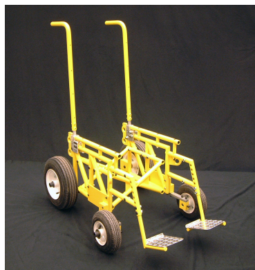
Figure 2.17 - Surrogate wheelchair frame (SWCF) used in tests to evaluate front- and rear-impact restraint systems to evaluate restraint systems in both front and rear impacts
