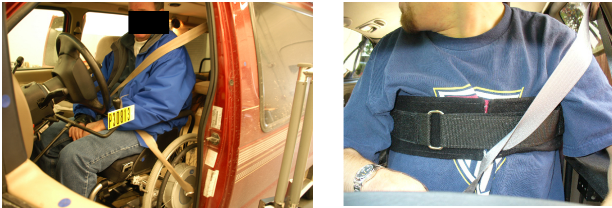
Figure 2.13 - Photos showing typical positioning of the shoulder belt nearly off (left) or completely off (right) the driver’s outboard shoulder
