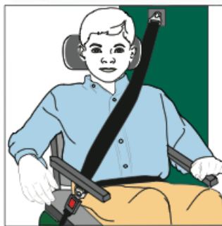
Good shoulder belt positioning over the center of the shoulder and chest
