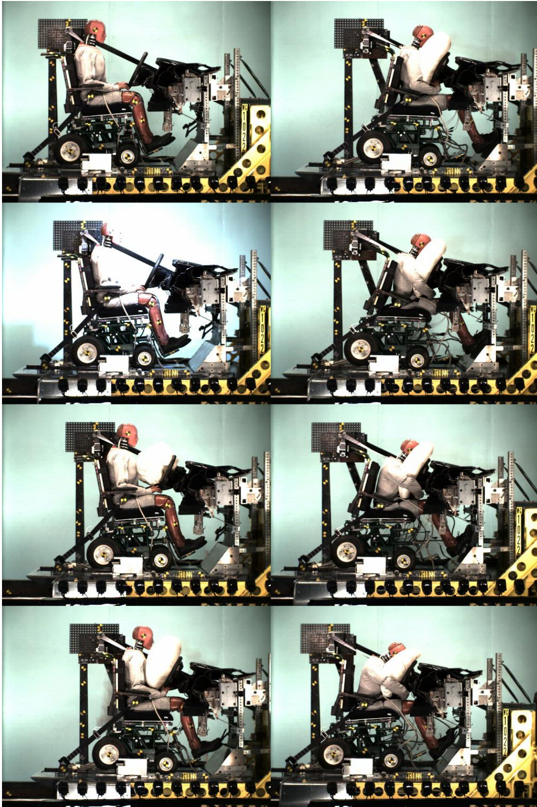
Figure 3.4 – Time-sequence frames from the side-view high-speed video from Test No. WC1022 with good belt fit and 12-ms air-bag deployment time, showing midsize-male ATD kinematics and interaction with the air bag
