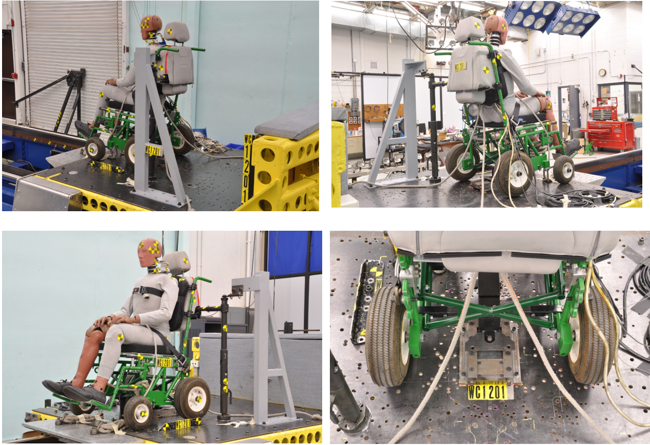
Figure 2.64 - Photos showing the setup of SWCF and midsize-male ATD for the first rear-impact sled test of the deployable Swedish head-and-back restraint system
