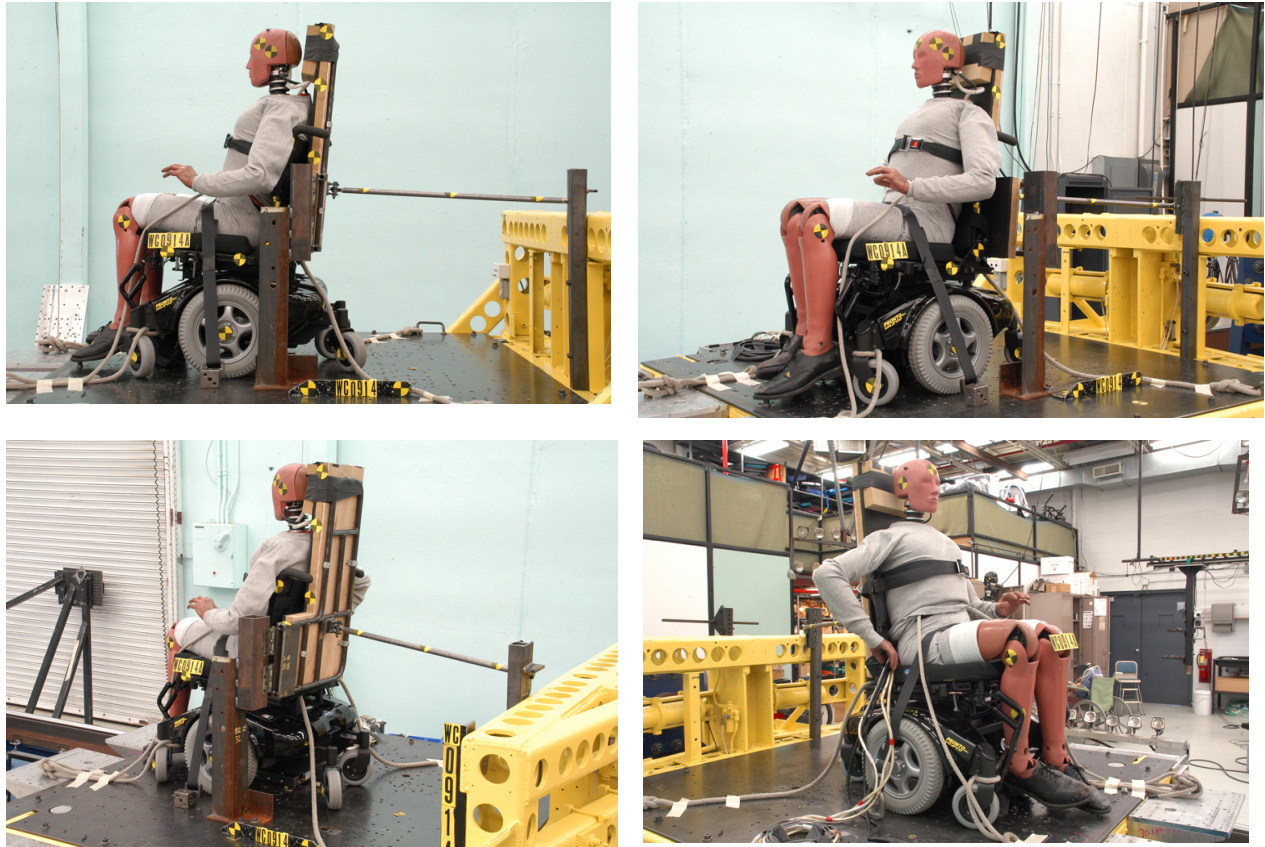
Figure 2.61 - Post-test photos of the second rear-impact sled test of a BME student-designed vehicle-mounted head-and-back restraint
