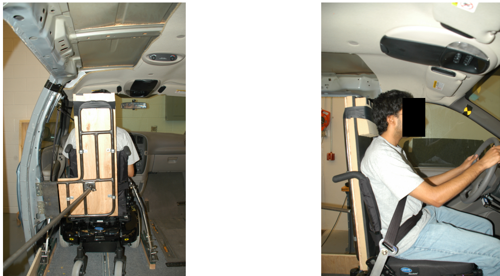
Figure 2.58 – Early prototype of the BME student-designed deployable vehicle-mounted head-and-back restraint in the deployed position behind a student seated in a wheelchair
