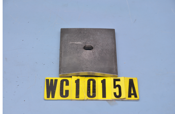
Figure 2.45 - Post-test photos for the sled test of Figure 2.44 showing the degree of plastic deformation of the 7.94-mm (5/16") thick hot-rolled steel plate on the right
