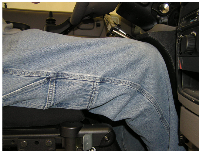
Figure 2.31 - Position of the right knee relative to a prototype contoured close-proximity knee restraint in the static minivan buck
