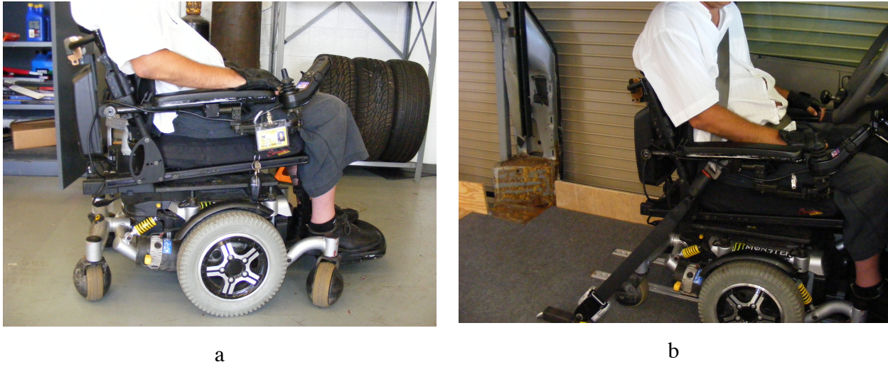
Figure 2.55 - Power wheelchair retrofitted with open-front cantilevered arm supports (a) and driver using a passive lap/shoulder belt with the seat-belt deployment system showing good fit of the lap belt low and in contact with the pelvis (b)
