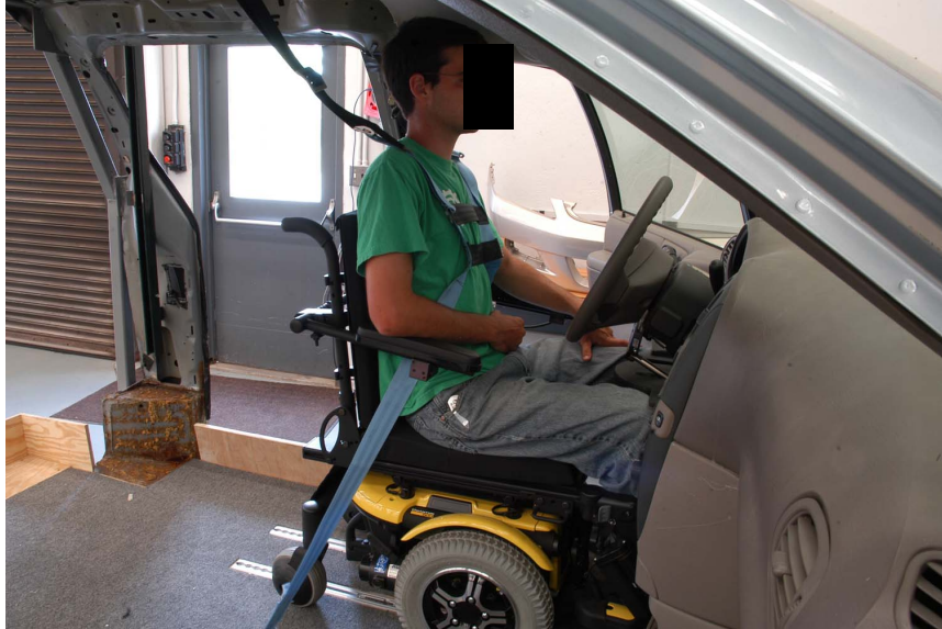
Figure 2.32 - A member of the UMTRI design team evaluating a prototype close-proximity knee restraint in the static minivan buck with a passive shoulder harness to provide upper-torso restraint
