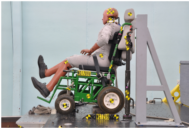
Figure 2.71 - Post-test photos from the third rear-impact test of the modified Swedish deployable vehicle-anchored head-and-back restraint system
