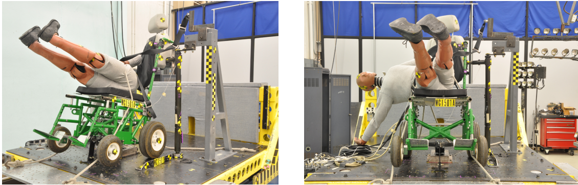
Figure 2.78 - Post-test photos of the Swedish manufacturer's modified design of the deployable vehicle-anchored head-and-back restraint system
