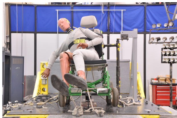
Figure 2.72 - Post-test photos from the fourth rear-impact test of the modified Swedish deployable vehicle-anchored head-and-back restraint system
