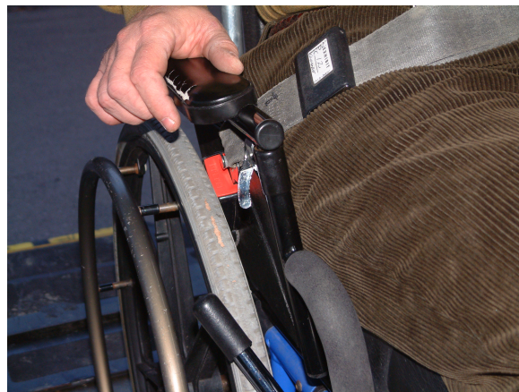
Lap-belt buckle with end-release button located close to rim of left wheelchair wheel
