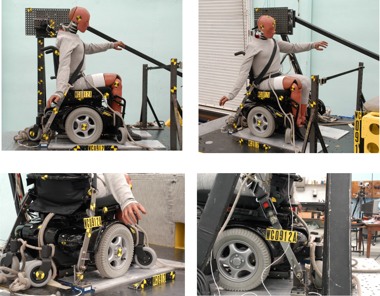
Figure 2.28 - Photos of the wheelchair and ATD following the third 48-kph, 20-g frontal-impact test of the prototype pivoting-bar lap/shoulder belt restraint system
