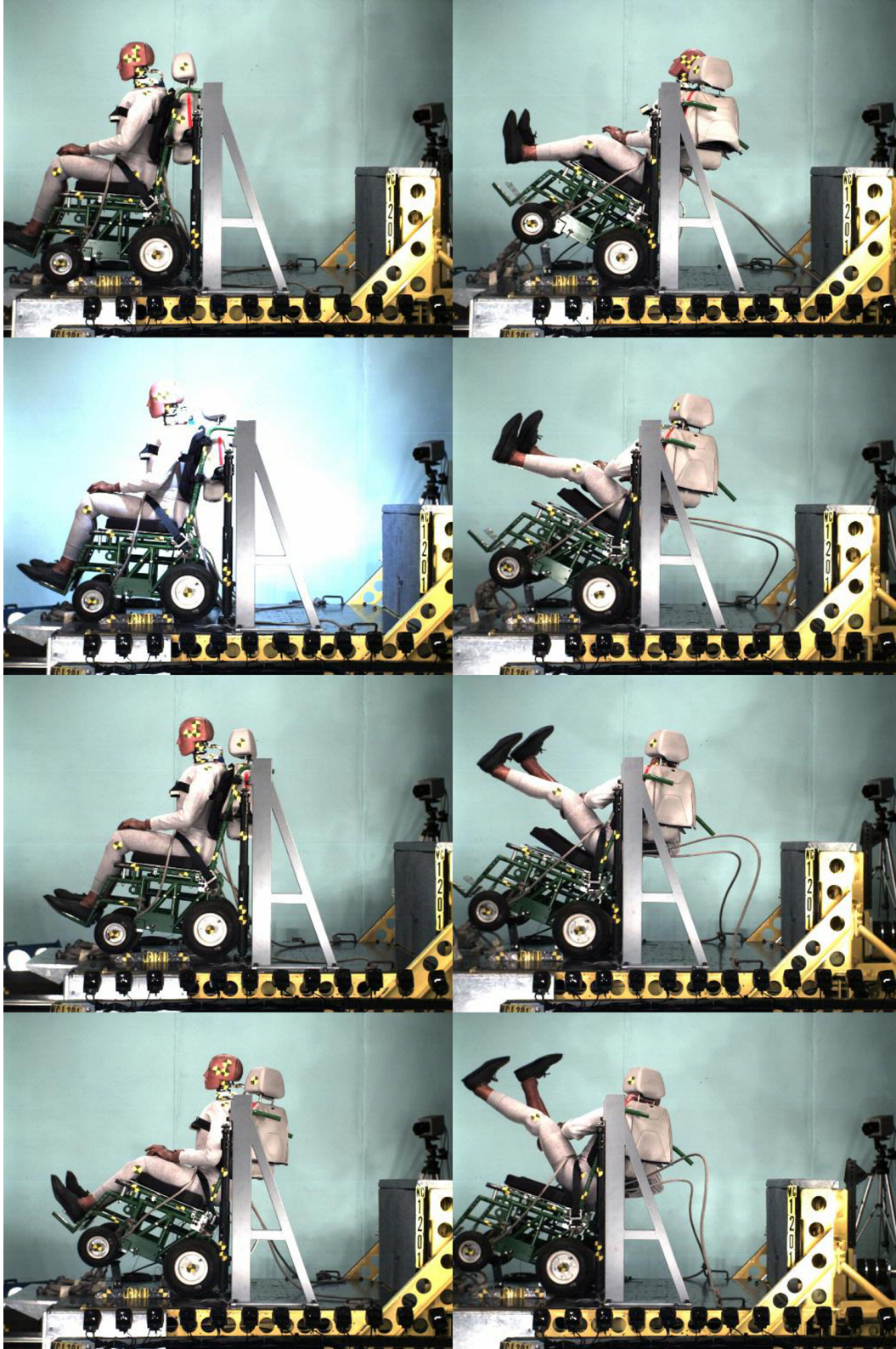
Figure 2.66 – Time-sequence photos from the side-view high-speed digital video of the first rear-impact sled test of the deployable Swedish vehicle-anchored head-and-back restraint system – note the rearward rotation of the SWCF
