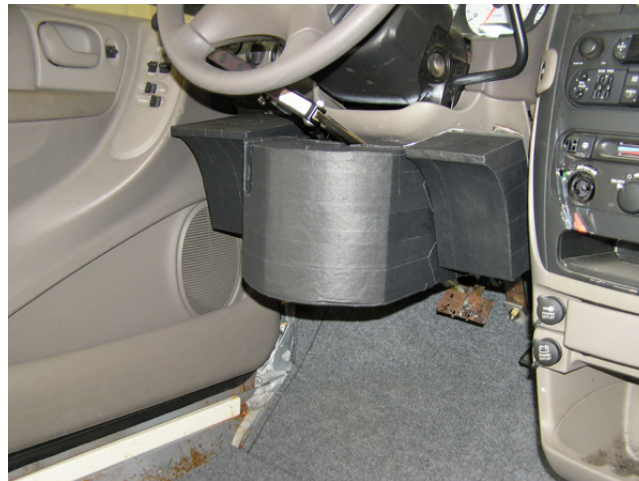
Figure 2.30 – Photo of a prototype close-proximity knee restraint installed in the static minivan buck
