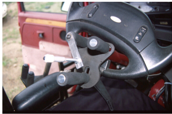
Tri-pin attached to lower steering-wheel rim
