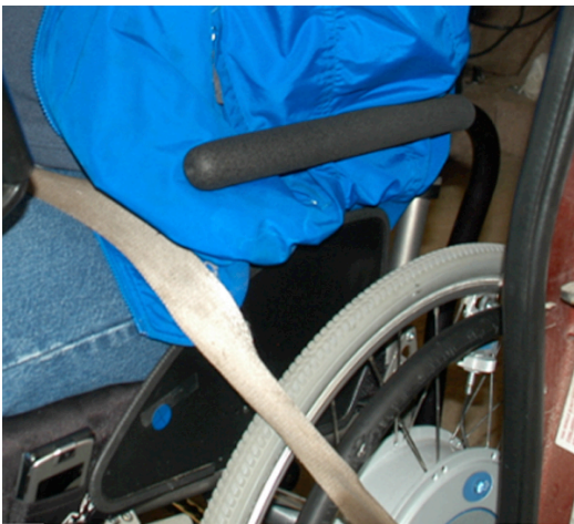
wheelchair with open-front arms supports
