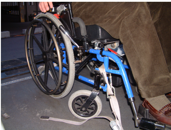
Lap-belt buckle with end-release button located close to rim of left wheelchair wheel
