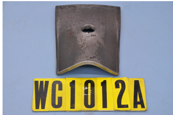
Figure 2.46 - Post-test photos showing plastic deformation of a 6.35-mm (1/4") thick hot-rolled steel plate still installed in the SDSD (left) and after removal from the SDSD (right)
