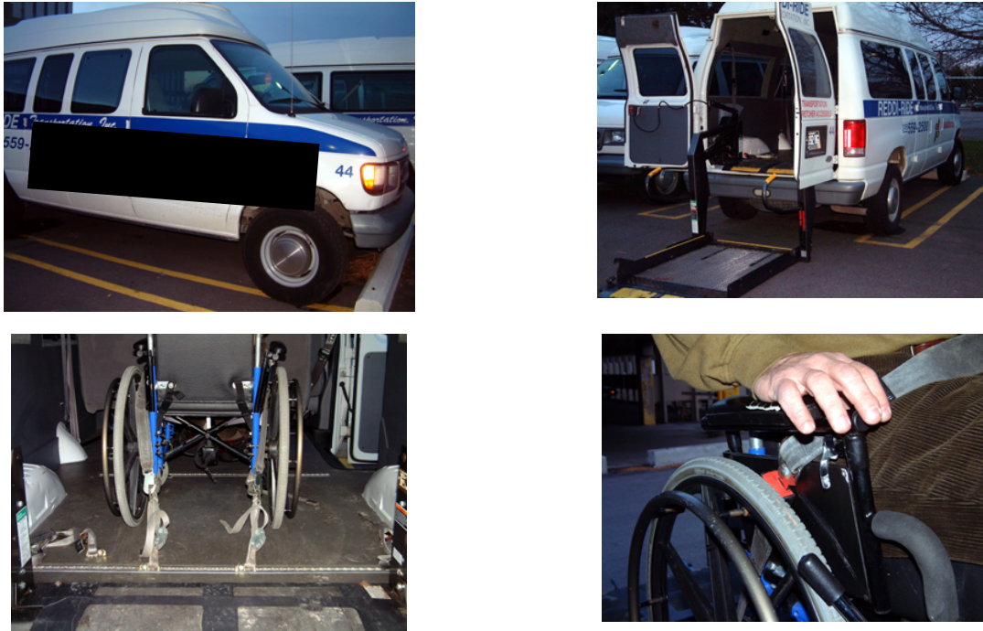
Figure 1.3 - Paratransit van similar to a van from which a lap/shoulder-belt restraint male passenger seated in a properly secured manual wheelchair was ejected during a four quarter-turn rollover due to contact of the buckle release button by the rim of the wheelchair wheel.
