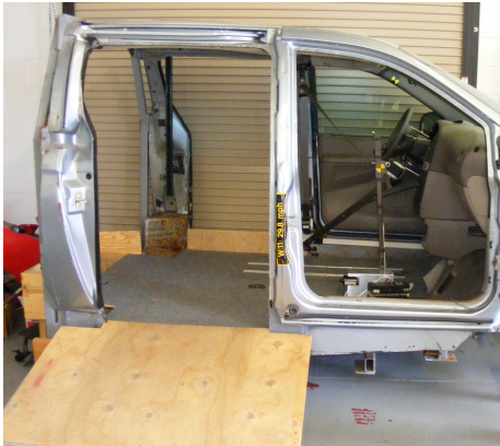
Figure 2.14 -Minivan buck in UMTRI high-bay laboratory with rear-entry and side-entry ramps used for wheelchair driver ingress and egress to evaluate prototype restraint-system designs
