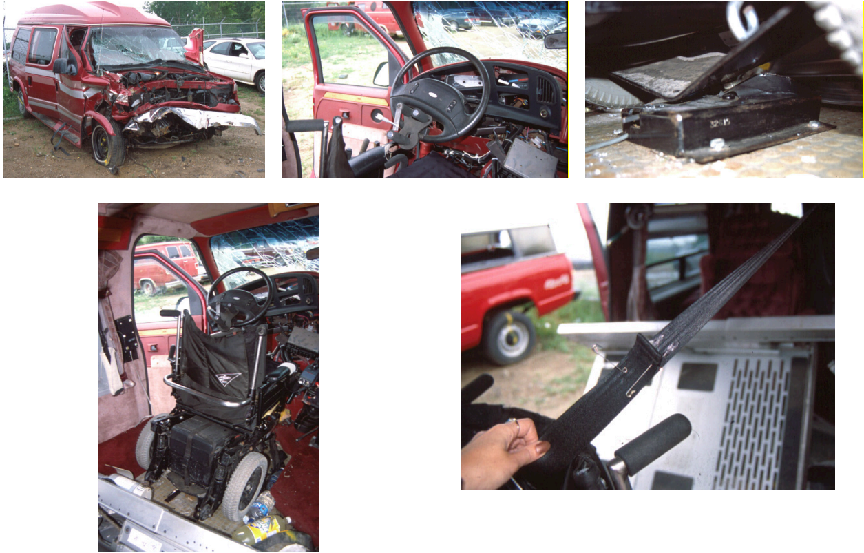
Figure 1.2 - Exterior and interior photos of a full-size van operated by a driver seated in a power wheelchair who sustained fatal chest and abdomen injuries in a severe frontal crash
