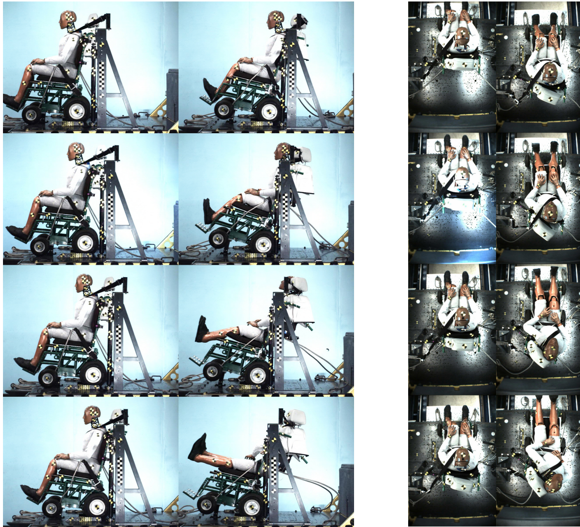
Figure 2.79 - Side-view (left) and overhead (right) time-sequence frames from high-speed videos for the rear-impact sled test of the Swedish manufacturer's modified design of the deployable vehicle-anchored head-and-back restraint system
