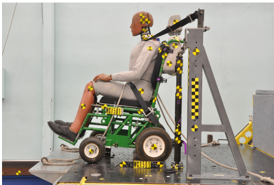
Figure 2.77 - Pre-test photos of the manufacturer’ revised design of the Swedish deployable vehicle-anchored head-and-back restraint system
