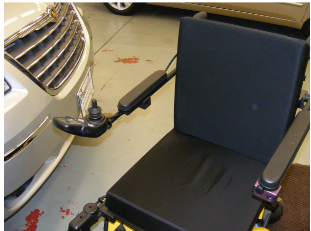
wheelchair with open-front arm supports
