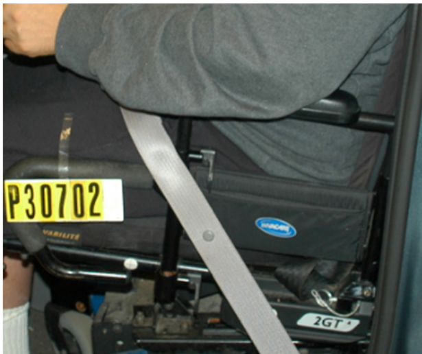
power wheelchair with closed desk-type arm supports
