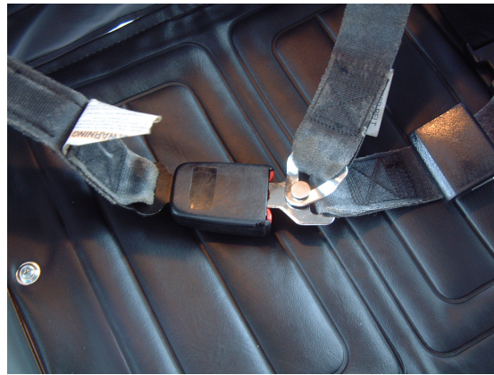
Lap-belt buckle with lower end of shoulder belt attached
