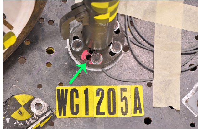
Figure 2.70 - Broken plastic drive nut (upper part of photo on left) on screw-motor actuator and slippage in curved slots at the base of the Swedish head-and-back restraint post (right) that were significant contributors to the poor performance of the Swedish deployable vehicle-anchored head-and-back restraint system in the second sled test
