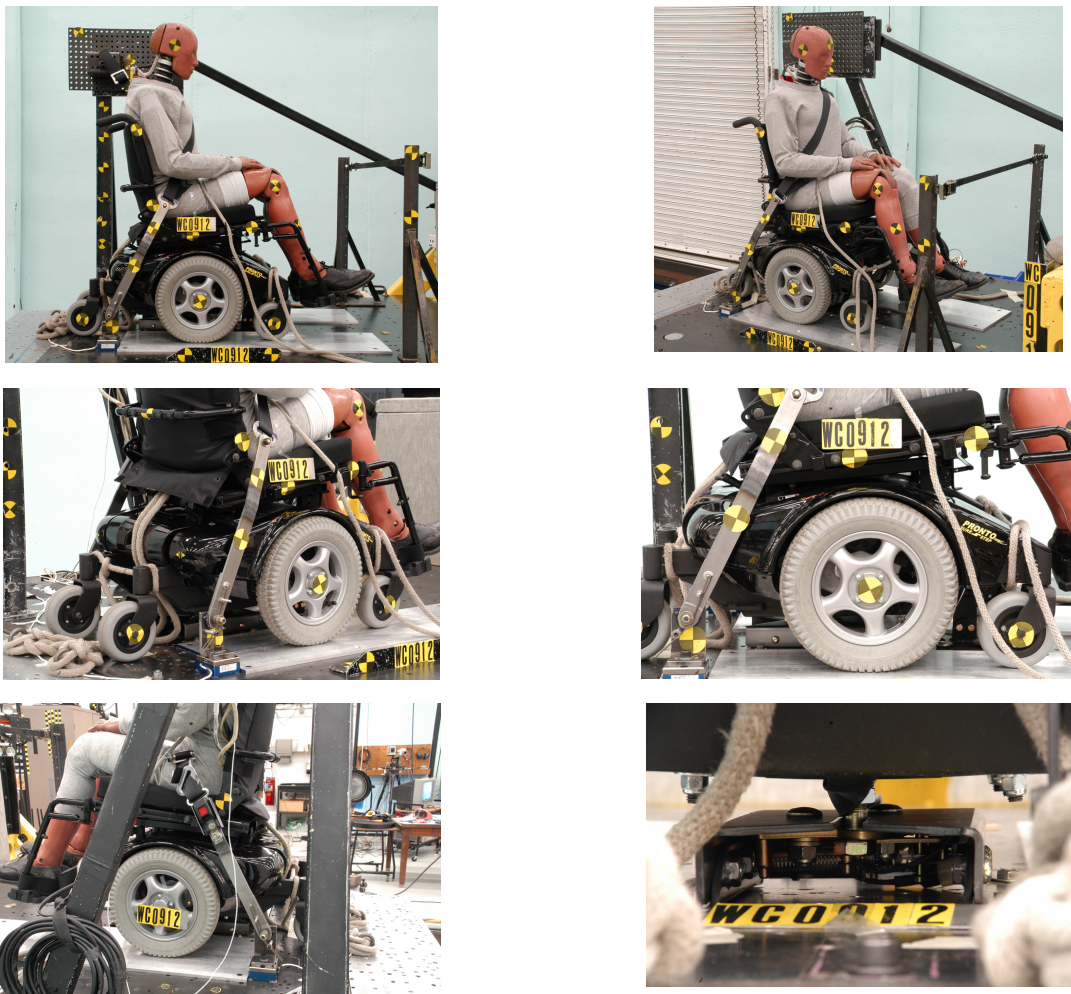
Figure 2.26 -Photos of the prototype pivoting-bar lap/shoulder belt restraint system prior to conducting the third and final 48-kph, 20-g frontal sled-impact test
