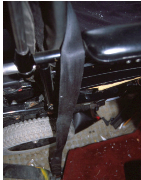
Routing of 2-pt shoulder belt over WC arm support
