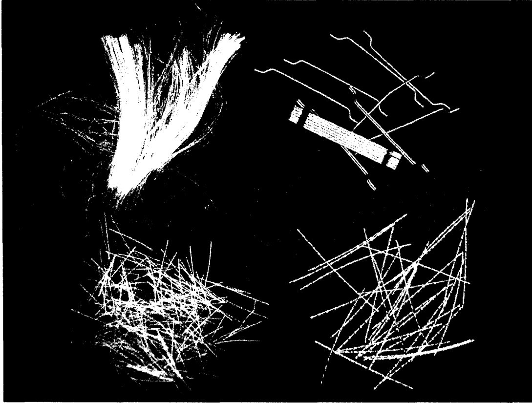
Figure 3.1 Fibers used in this study: (a) Spectra (upper left); Steel Hooked (upper right); PVA 13 (lower left); Rectangular Torex (lower right)
